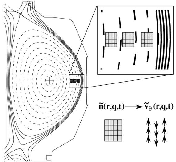
FIG. 1. Experimental configuration of BES channels for this experiment-4x4 grid, measuring a 3.6 (radial) x 5.0 (poloidal) cm region at the outboard midplane and radially scanned, as shown in inset. Flow measurements are derived via TDE analysis of 2D measurements, illustrated in lower inset.
