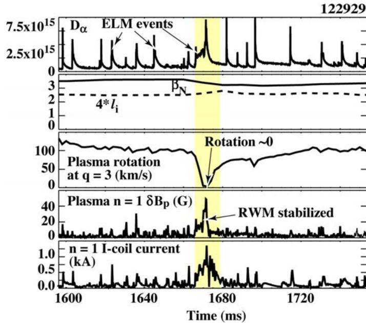
FIG. 5. Prompt response by the RWM feedback system using the I-coil to a mode growth following a large ELM and fast rotation slowdown, allows recovery of the plasma rotation and sustinment of  $\beta_N > 4l_i$ .
