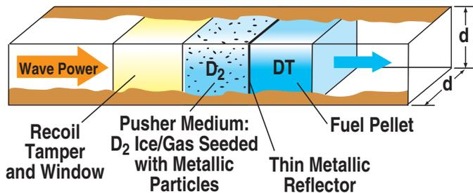
Fig. 2. Composite pellet structure.
