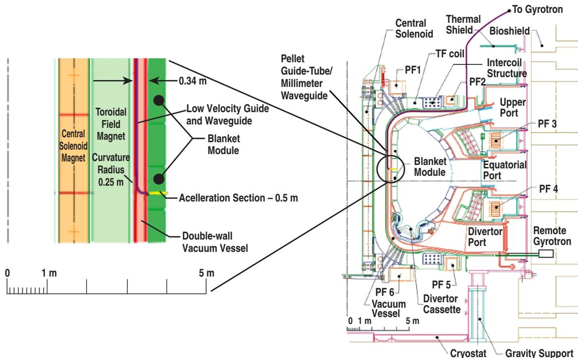
Fig. 1. Poloidal plan view of ITER design; detail of acceleration region.
