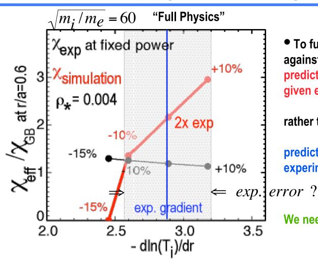
To fully test a stiff transport model against experiment, one must predict the temperature profile from given experimental power flows;
