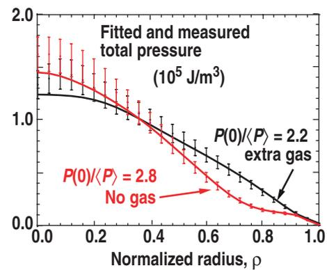
Fig. 2. Measured pressure profiles for discharges with and without extra gas puff to broaden the density and pressure profiles.
