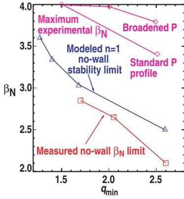
Fig. 3. Experimental and theoretical scaling of  $\beta_N$  with the minimum value of  $q$ .
