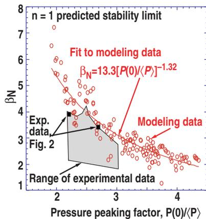
Fig. 1. Calculated ideal  $n = 1$  stability limit as a function of pressure peaking (circles). The scatter in points is a result of variation of discharge shape. The squares are the measured values for the discharges in Fig. 2.
