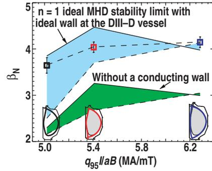
Fig. 4. Measured (squares)  $\beta_N$  for three discharges with varying shape. Higher values of  $q_{95} I/aB$  have stronger shaping. Shaded areas show the calculated ideal  $n=1$  limit where the shading represents the profile measurement uncertainties.
