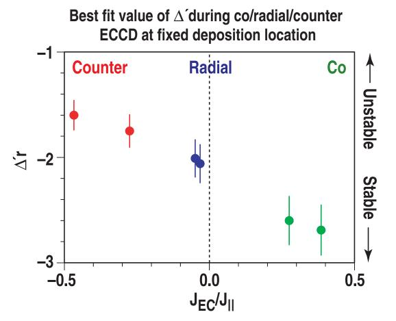
● Although △´ modification is significant, direct current drive in island is main reason for 2/1 tearing mode suppression
