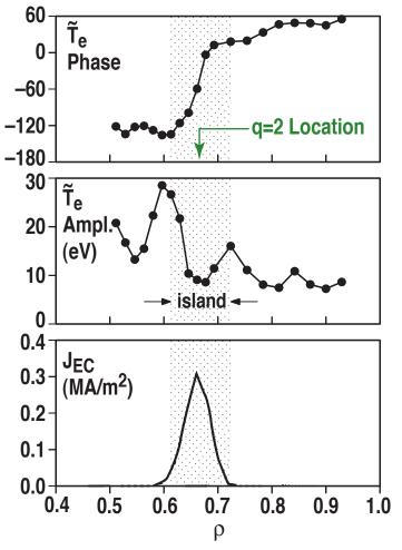
2/1 mode suppressed in hybrid discharge with  $\beta_N$  well above ITER baseline scenario
