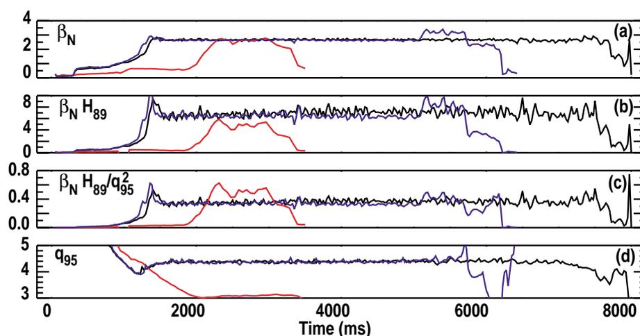
Fig. 1. Comparison of (a) normalized  $\beta$  ( $\beta_N$ ), (b) normalized performance ( $\beta_N H_{89}$ ), (c) the ignition figure of merit ( $\beta_N H_{89} / q_{95}^2$ ), and (d) the  $q_{95}$  in a conventional, low  $q$  discharge with two discharges at  $q_{95} \sim 4.5$ .
