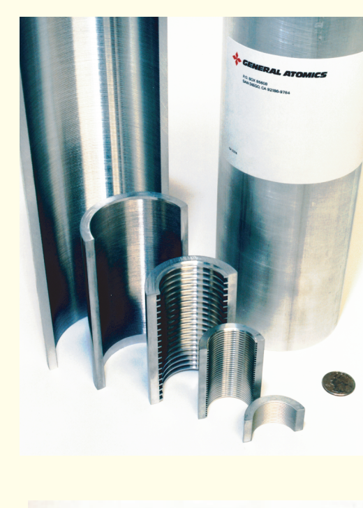
Step corrugated vacuum waveguide for various wavelengths
