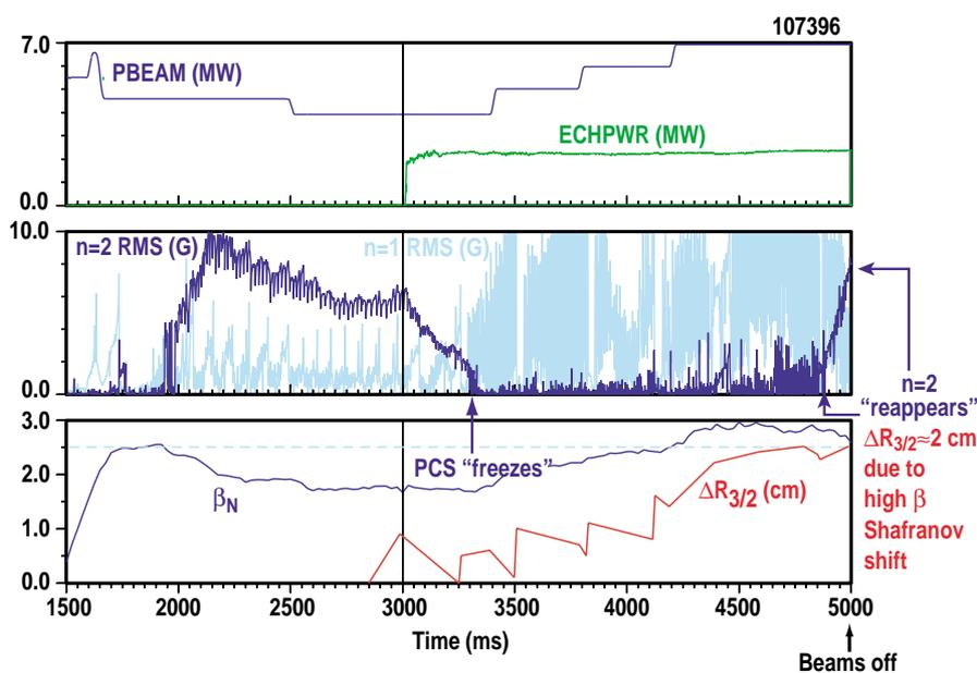
Fig. 1. Approximately 2.3 MW of ECCD is used to suppress an  $m/n=3/2$  NTM in discharge #107396 after which neutral beam power is raised to increase beta.  $\beta_N$  is increased by 55% (despite large sawteeth and fishbones). The NTM reappears because the Shafranov shift has moved  $q=3/2$  about 2 cm off the optimum ECCD location. Note that there is no further PCS position optimization once the NTM has been suppressed.
