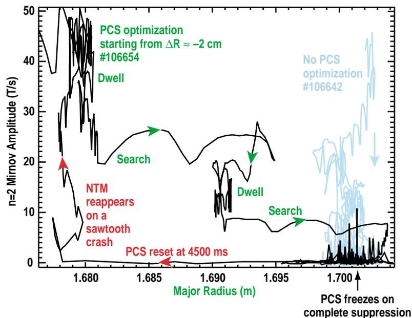
Fig. 2. Trajectory of  $n=2$  Mirnov amplitude versus plasma major radius with (#106654) and without (#106642) real-time control of optimum rigid plasma position for ECCD suppression ( $m/n=3/2$  NTM, three gyrotrons for 1.5 MW injected from 3000 to 4800 ms).
