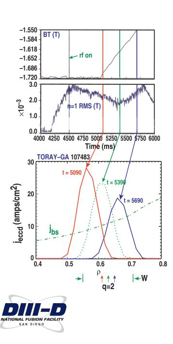
Sweeping B<sub>T</sub> moves j<sub>eccd</sub> past q=2 island ★ j<sub>eccd</sub> > j<sub>bs</sub> is satisfied (TORAY-GA) 4 gyrotrons for  $\approx$  2 MW injected **ECH** f = 110.0 GHz facet ang = 12.0 deg tilt ang = 56.0 deg NN +
