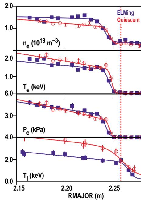
FIG. 5. Typical edge profiles for  $n_e$ ,  $T_e$  and  $p_e$  for ELMing and quiescent phases of same discharge are similar. In particular, gradients in transport barrier are similar.  $T_i$  is higher in quiescent phase. Vertical dashed lines show locations of separatrices at two times.
