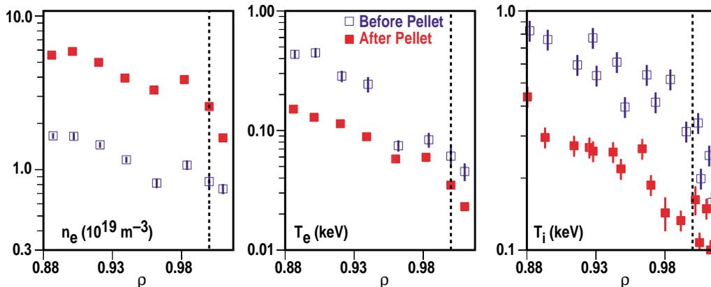
FIG. 1. Edge  $n_e$  rises by about factor of 3 and edge  $T_e$  and  $T_i$  decrease by about 50% from before pellet injection (18 ms before H-mode transition) to after pellet injection (6 ms before H-mode transition). Separatrix shown by vertical dashed lines.
