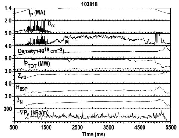
FIG. 4. Typical waveforms for quiescent mode show that, after a short ELMing phase ends ( $\approx 1600$  ms), confinement parameters reach steady-state. These include density, radiated power, confinement enhancement factor, core  $z_{\text{eff}}$  normalized toroidal beta and pressure gradient in H-mode barrier. Amplitude of magnitude fluctuations, shown by  $|B|$  changes character after end of ELMs and indicates presence of MHM-mode.
