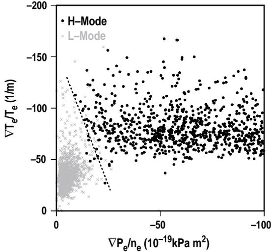
FIG. 2. Operational space diagram showing that  $\nabla T_e/T_e$  and  $\nabla P_e/n_e$  distinguish very well between L-mode and H-mode. Data are drawn from scans of density, current and toroidal field and from discharges with PIH-modes. Dashed line shows approximate division between the two states. Of the 2000+ points used for the figure, more than 99% are classified correctly by the dashed line.
