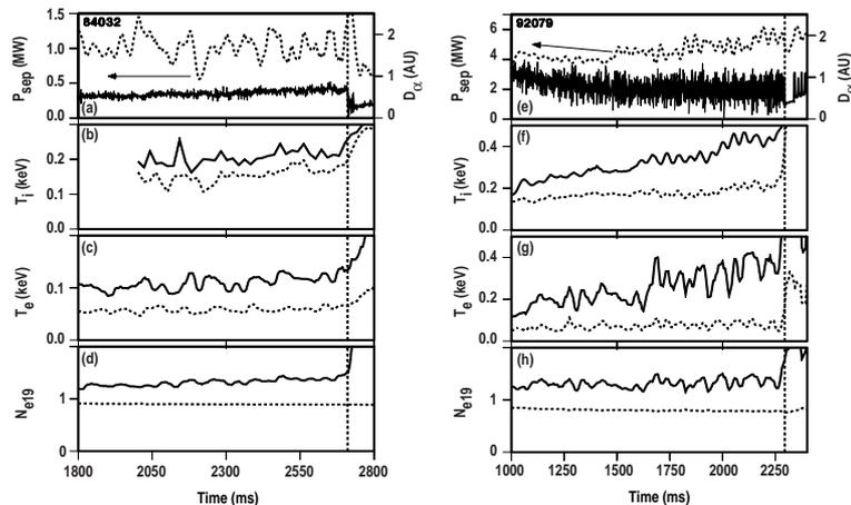
**Figure 2.** Panels (a-d) and (e-h) show waveforms for discharges in which the H-mode power threshold was respectively close to and much larger than the Ohmic power in absence of auxiliary heating. Vertical dashed lines indicate time of L-H transition.  $P_{sep}$  is power flow through the separatrix.  $N_{e19}$  is electron density in units of  $10^{19} \text{ m}^{-3}$ . In panels (b-d) and (f-h), solid lines show data at density knees and dashed lines show data at density symmetry points.
