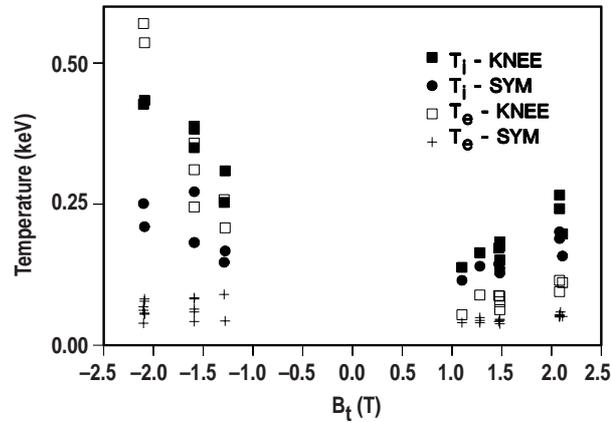
**Figure 3.** Edge temperatures as function of toroidal magnetic field and direction. Positive (negative) magnetic field corresponds to normal (reversed) direction of  $B_t$  and the  $\nabla B$  drift is in the favorable (unfavorable) direction.
