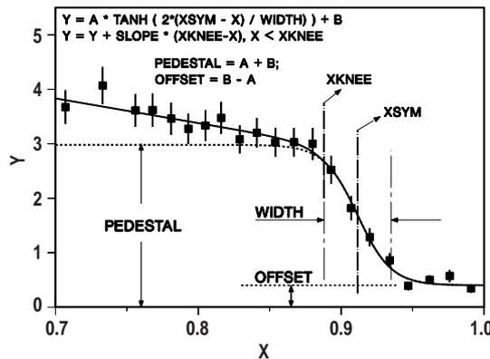
**Figure 1.** Definition of hyperbolic tangent fit to edge profile. The solid squares are measurements of some quantity Y as a function of some spatial coordinate X. The solid line is the fit to the data of the hyperbolic tangent function plus a constant offset term plus a linear term for points inside the knee of the profile.
