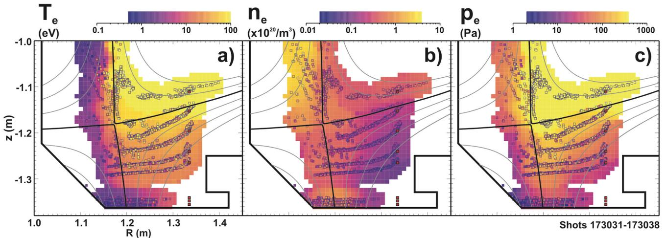
FIG. 9. Composite 2D constructions of (a)  $T_e$ , (b)  $n_e$ , and (c)  $p_e$  based on measurements as the divertor leg is swept past the measurement locations shown as red squares at  $R = 1.335 \text{ m}$ . The data is then mapped to magnetic flux surfaces and displayed at a fixed x-point location.
