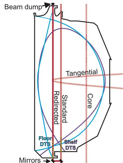
FIG. 1. Location of the laser beams for Thomson scattering measurements in DIII-D. Also shown are the standard shelf Divertor Thomson Scattering (DTS) measurement locations and the new floor DTS locations.
