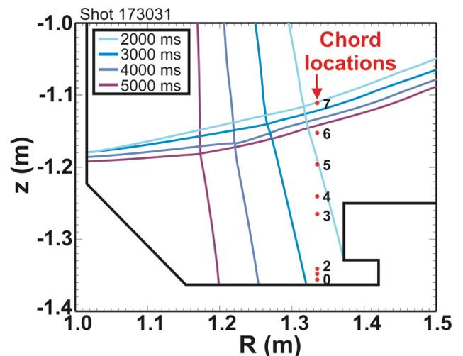
FIG. 6. Reconstructed separatrix locations relative to the floor divertor Thomson scattering (DTS) chord locations at various times during the x-point sweep of shot 173031.
