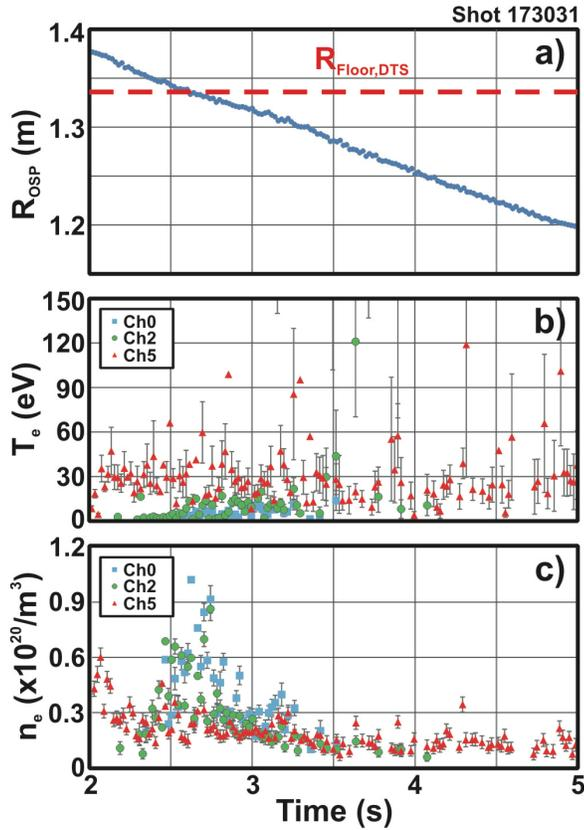
FIG. 7. Time evolution of (a) the variation of the outer strike point ( $R_{OSP}$ ) and the floor DTS ( $R_{FLOOR\_DTS}$ ) location, (b)  $T_e$  and (c)  $n_e$  for three of the floor divertor channels
