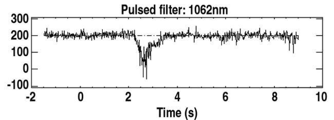
FIG. 5. Raw data in digitizer counts of the Thomson scattered signal from the lowest floor divertor channel for shot 173031. The signal is from the 1062 nm wavelength channel and light produces negative going signals. The dashed line represents the no-light signal level. The laser starts firing at -1.5 sec and the plasma discharge starts at 0.0 sec.
