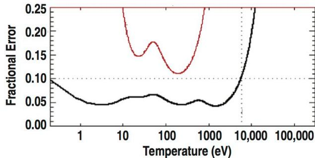
FIG. 4. Calculated expected fractional  $T_e$  measurement error from an 8 channel polychromator (black) compared to a previous 6 channel polychromator (red). The addition of the 1067 nm filter extends the range to less than 1 eV, and an 800 nm filter increases the range to over 8 keV.
