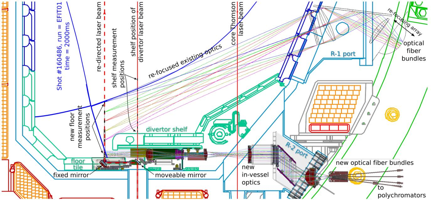
FIG. 2. Schematic of the lower divertor showing the re-directed laser beam to the floor region, in-vessel relay optical elements, and the existing optics of the current system with adjustable focus. The separatrix of a high-triangularity plasma discharge is overlain.
