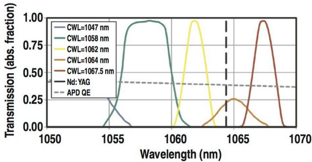
FIG. 3. Interference filter transmission of filters on both the long and short wavelength sides of the laser line (vertical dashed line).
