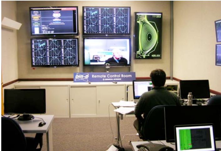
Fig. 7-7. The existing DIII-D Remote Control Room used for KSTAR operations in 2011. Five large TVs face the scientific staff and 6 smaller 24 in. monitors display plasma control quantities (right).
