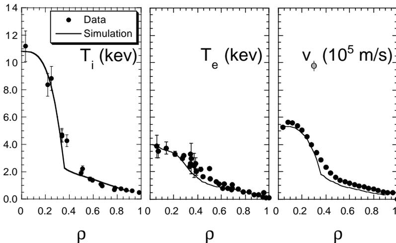
FIG. 2. Ion temperature, electron temperature, and toroidal velocity profiles from the GLF23 model at the end of the simulation compared against experimental data for #84736.
