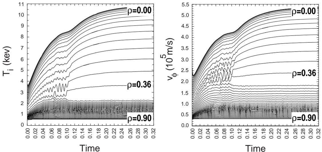
FIG. 1. Time evolution of ion temperature and toroidal velocity predicted by the GLF23 model for DIII-D NCS discharge #84736 at 1.30 s. Values are shown at various radii with an equal spacing in normalized toroidal flux of 0.02.
