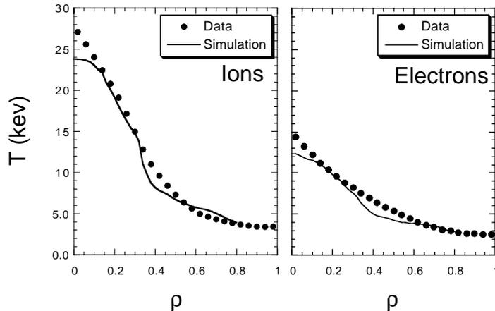
FIG. 3. Steady-state ion and electron temperature profiles from the GLF23 model compared against experimental data for JET OS discharge #40847 at 46.86 s.
