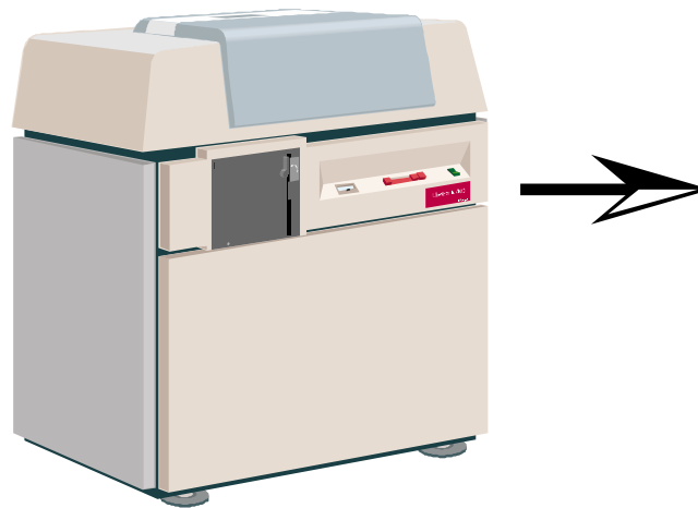
HP Magneto-optical 600fx 620 GB from 238 platters 2.6 GB/platter, 6 drives
