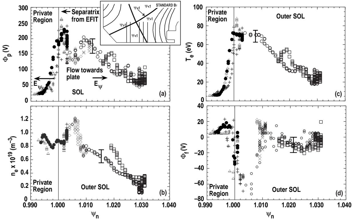
FIG. 1. Measured profiles of (a)  $\Phi_p$ , (b)  $n_e$ , (c)  $T_e$ , and (d) floating potential,  $\Phi_f$ , in the outer divertor leg as a function of  $\psi_n$  for standard  $B_T$  direction. Inset shows probe trajectories schematically in these ELMing H-mode plasmas.
