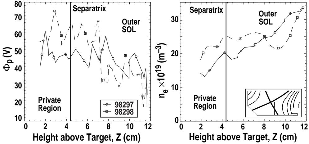
FIG. 3. Measured profiles of (a)  $\Phi_p$  and (b)  $n_e$  vs. height above target during PDD conditions for standard  $B_T$ .
