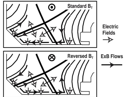
FIG. 4. Schematic of  $\mathbf{E}$  and  $\mathbf{E} \times \mathbf{B}$  directions in the divertor for standard and reversed  $B_T$ .
