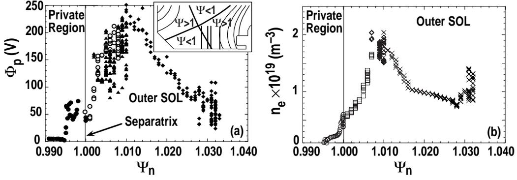
FIG. 2. Measured profiles of (a)  $\Phi_p$  and (b)  $n_e$  for reversed  $B_T$ , attached, H-mode plasmas.
