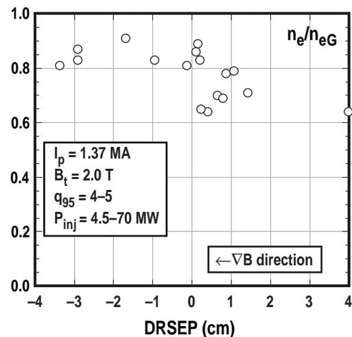
Fig. 4. The H-mode density limit changes measurably between  $DRSEP = 0$  and 1.5 cm. The density is normalized to the Greenwald density limit.
