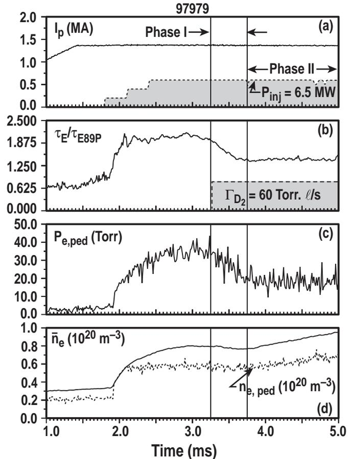
Fig. 3. Deuterium gas is injected into a lower SN divertor plasma, starting at  $t = 3.25$  s.  $DRSEP = -3.7$  cm. Phase I: Electron energy confinement degrades with little rise in density. Phase II: Energy confinement is stable and density rises.
