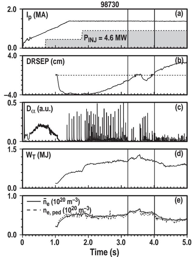
Fig. 2. The “dynamic” scan in DRSEP shows that small shifts away from  $DRSEP = 0$  result in SN behavior. There was some variation in  $q_{95}$  between  $t = 2.0$  and  $5.0$  s; between  $t=3.0$  and  $4.2$  s,  $q_{95} = 4.7$ – $5.1$ .
