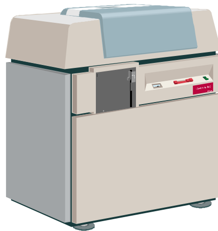
HP Magneto-optical 600fx 620 GB from 238 platters 2.6 GB/platter, 6 drives
