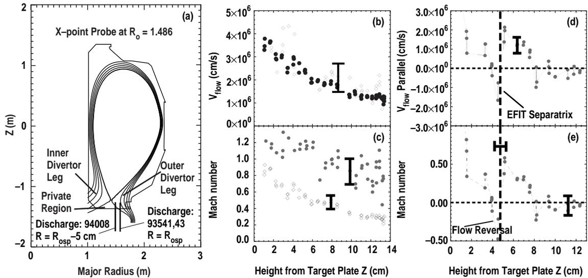
Fig. 1. The plasma and divertor geometry and the probe paths are shown. The path labeled  $R_{osp}-5$  cm crosses the separatrix and the path labeled  $R_{osp}$  enters the SOL directly (a) Measurements of ion velocity (b) and Mach number (c) are obtained by the probe for attached (diamonds) and detached (circles) discharges. We also show the measurements of flow velocity (d) and Mach number (e) obtained at the path crossing the separatrix, and showing flow reversal.
