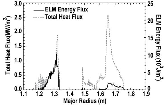
Fig. 2. ELM divertor energy deposition profile for ASDEX-Upgrade.
