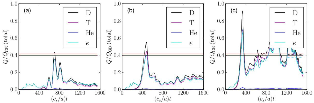
Figure 2: GYRO simulations at  $r/a = 0.4$ . Plot (a) shows simulation at nominal TGLF gradients  $(z_i, z_e) = (1.130, 1.226)$ , (b) at  $(1.243, 1.349)$  and (c) at  $(1.356, 1.471)$ . Horizontal lines are nominal TGLF electron (red) and total ion (black) fluxes.
