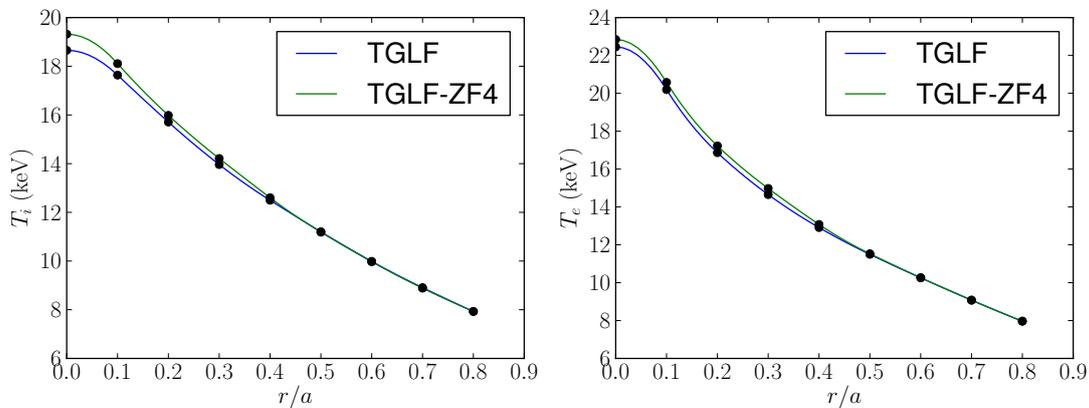
Figure 3: Profile modification using TGLF-ZF4 (i.e., zonal-flow effects added to TGLF at  $r/a = 0.4$ ) compared with baseline TGLF prediction.
