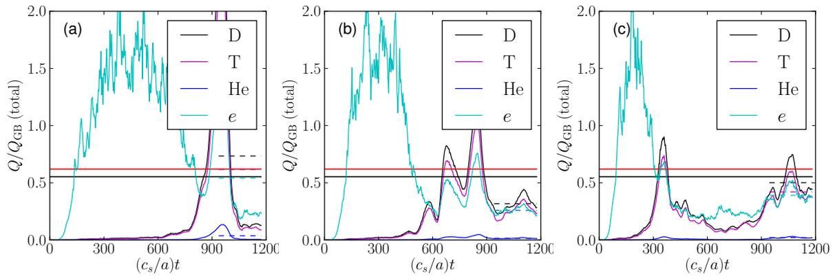
Figure 4: GYRO simulations at  $r/a = 0.5$ . Plot (a) shows simulation at nominal TGLF gradients  $(z_i, z_e) = (1.138, 1.110)$ , (b) at  $(1.252, 1.221)$  and (c) at  $(1.366, 1.442)$ . Horizontal lines are nominal TGLF electron (red) and total ion (black) fluxes.
