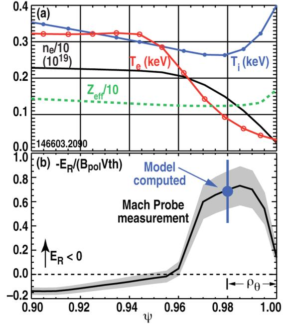
Fig. 1. (a) Edge profiles shortly after L-H transition. (b) Mach probe measure of  $E_r$  plotted as  $E_r/B_{\text{pol}}V_{\text{th}}$  and the model computed value for balance of thermal return and loss currents. The  $D+$  poloidal gyroradius,  $\rho_\theta$ , is  $\sim 7$  mm.
