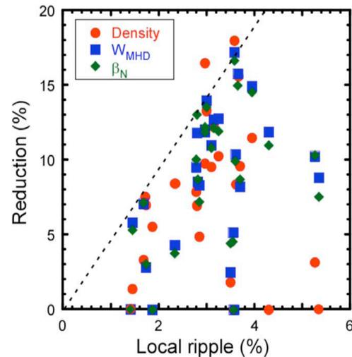
Fig. 4. Percent reduction in the line averaged electron density, plasma stored energy, and normalized  $\beta$  versus the local TF+TBM mock-up ripple in DIII-D. The dashed line indicates a rough maximum reduction versus ripple.
