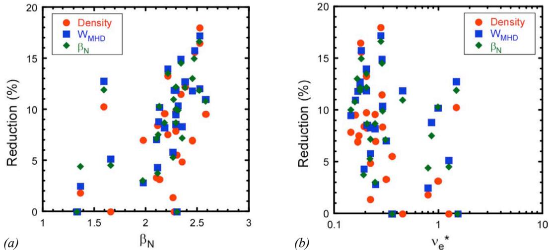
Fig. 5. (a) Percent reduction in line averaged electron density, plasma stored energy, and normalized  $\beta$  vs normalized  $\beta$  during the mock-up TBM showing that the confinement reduction increases with increasing  $\beta_N$ . (b) The same quantities vs the electron collisionality at the top of the edge pedestal showing no clear dependence on  $\nu_e^*$ .
