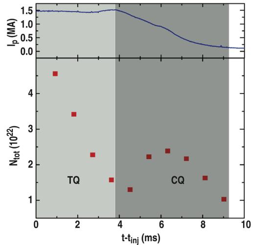
Fig. 2. Plasma current (upper) and  $N_{\text{tot}}$  (lower) during an SPI-induced shutdown with thermal energy content of 1600 kJ ( $t_{\text{inj}}$  being the injection time). The light shaded area shows the TQ phase and the dark shaded one the CQ phase.
