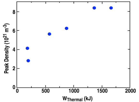
Fig. 1. Peak density observed after a shattered pellet injection as a function of the thermal energy content of the discharge.
