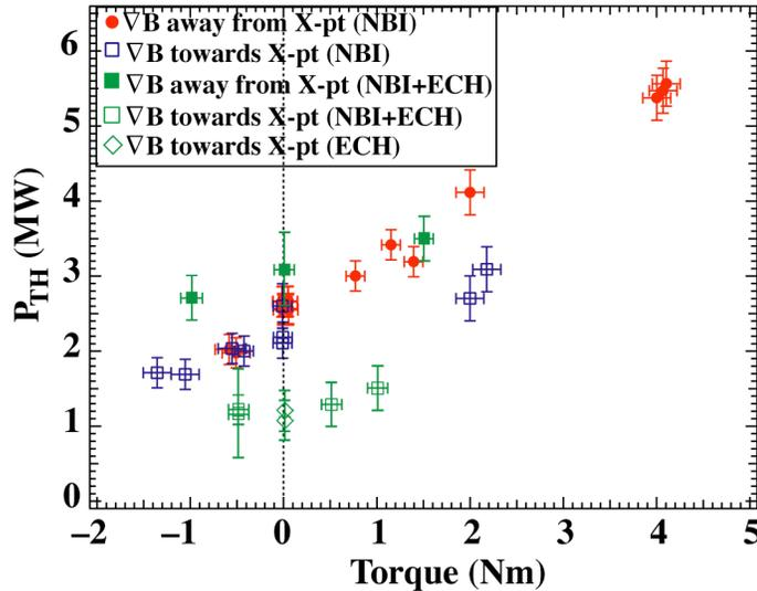
Figure 1. The H-mode threshold power as a function of the input torque from neutral beams. The dependence is shown for plasma discharges with the ion  $\nabla B$  drift away from the X-point (USN) and for plasmas with the ion  $\nabla B$  drive towards the X-point (LSN).
