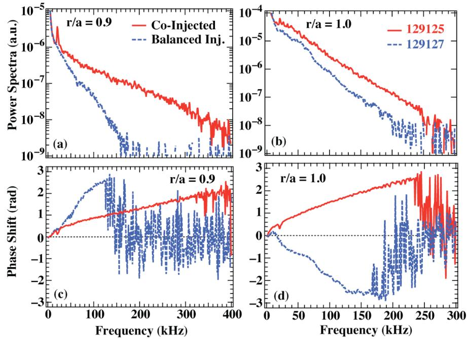
Figure 3. Density Fluctuation power spectra and phase for BES channels at two radial locations ( $r/a = 0.9$  and  $1.0$ ). (a) and (b) Density fluctuation power spectra at  $r/a = 0.9$  and  $1.0$ , respectively, for an all co-injection USN discharge (129125) and for a balanced injection USN discharge (129127). (c) and (d) phase shift at  $r/a = 0.9$  and  $1.0$ , respectively, between two poloidally separated measurements ( $\Delta Z = 1.2$  cm) for the same two discharges.
