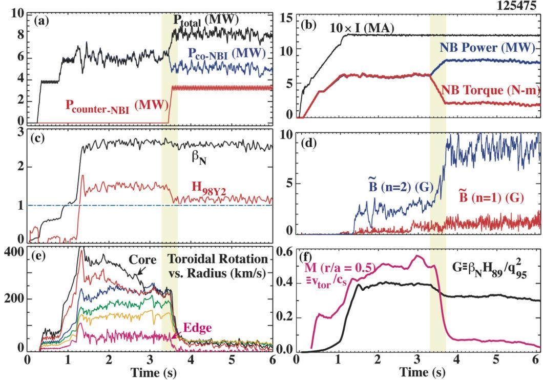
Fig. 1. Hybrid discharge quality  $\{\beta_N, H_{98Y2}, (f) G\}$  is maintained as core toroidal rotation (e) is decreased from  $M=0.5$  to  $M\sim 0.1$  (f) with counter neutral beam injection (a,b). A slight reduction in  $H_{98Y2}$  results in a 20% reduction in  $G$ . The benign  $n=3/2$  MHD mode suppresses sawteeth, and increases as the rotation decreases (d).
