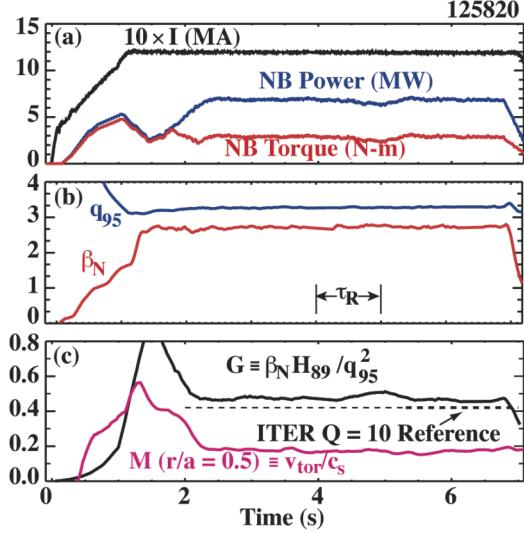
Fig. 2. An AI discharge where the central rotation is decreased with counter injection (a) at about 2 s. (b) The plasma  $\beta_N$  is maintained with neutral beam feedback, and  $q_{95} \sim 3.3$ . (c)  $G$  is maintained at a level greater than that projected for ITER operation at  $Q_{FUS} \sim 10$  (dotted line).
