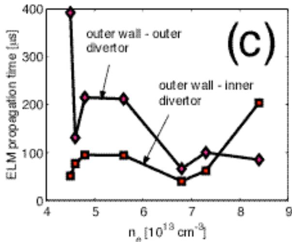
ELM radiated energy, peak emissivity and propagation time for different regions as a function of plasma density
