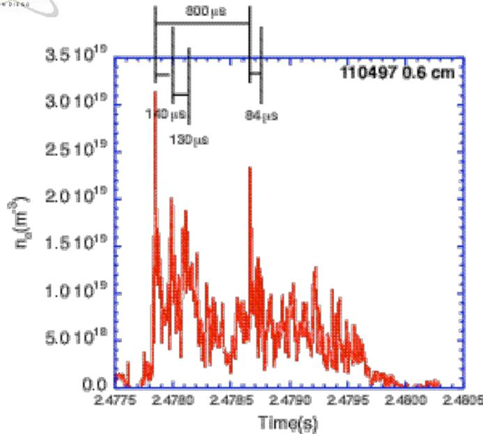
Perhaps an  $n=3$  structure (or multiple filaments) rotating with  $T=800 \mu$ s
