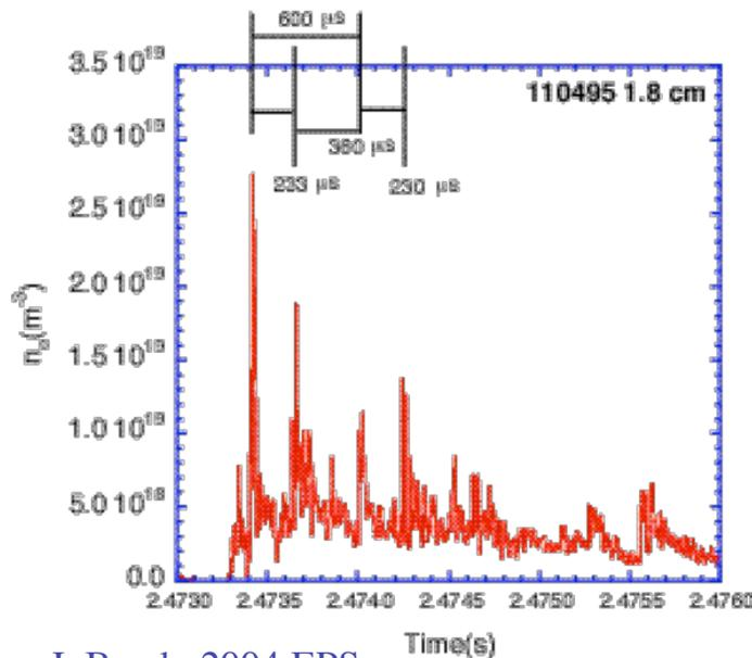
Perhaps an  $n=2$  structure (or multiple filaments) rotating with  $T=600 \mu$ s
