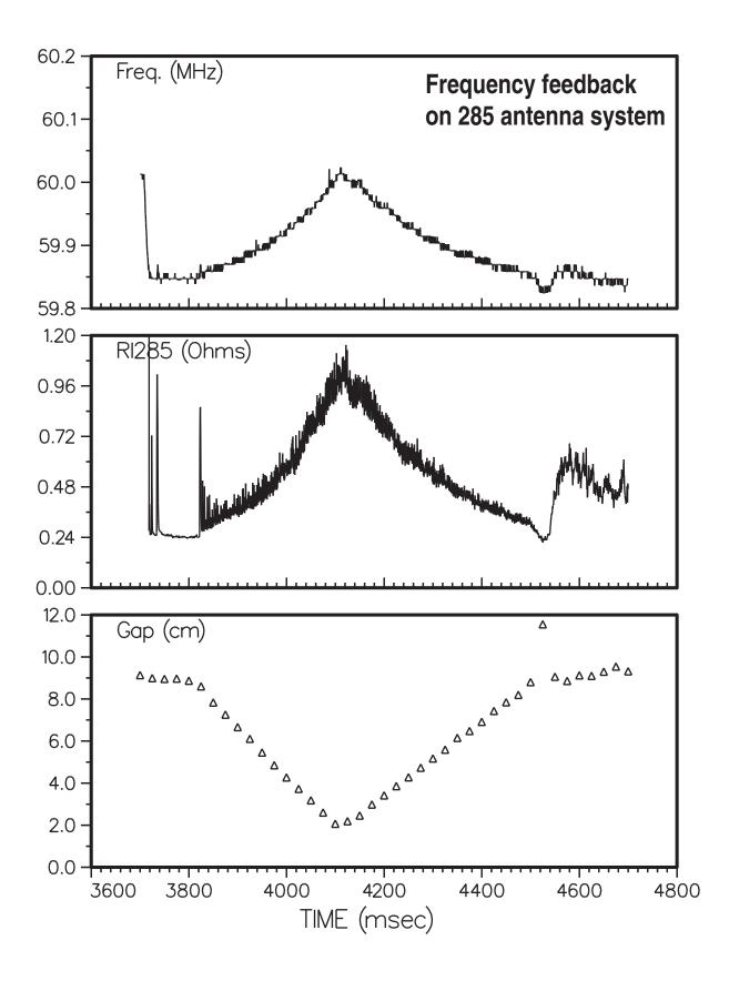
Antenna loading measured in dynamic gap ramps (between ELMs) is in reasonable agreement with predictions of a very simple model
