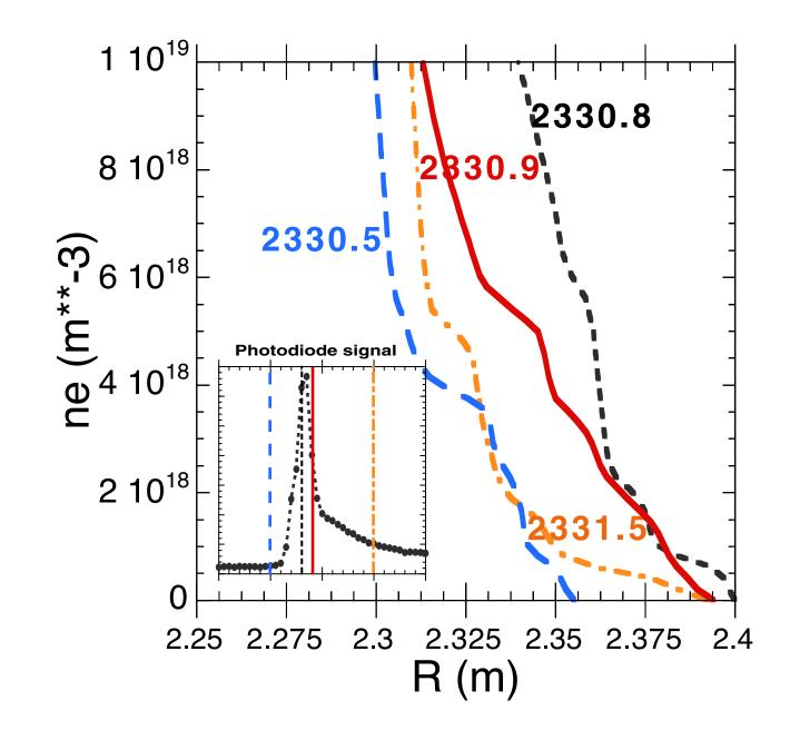
Edge density profiles measured with the FM reflectometry system during an ELM; outer gap of 8.3 cm
