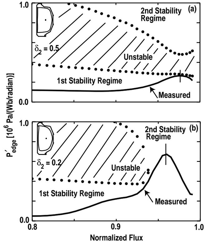
Fig. 1. Measured edge pressure gradient, and infinite- $n$  conventional ballooning stability boundaries (a) during high frequency ELMs in a high squareness ( $\delta_2 = 0.5$ ) discharge and (b) during low frequency ELMs in a moderate squareness case ( $\delta_2 = 0.2$ ).
