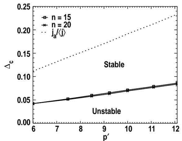
Fig. 4. Critical value of  $\Delta$  for instability to peeling modes, as a function of the pressure gradient, using model equilibria with squareness  $\delta_2 = 0.05$ ,  $n = 15, 20$ . Also shown is the normalized edge current ( $j_{a,d} / \langle j \rangle$ ).
