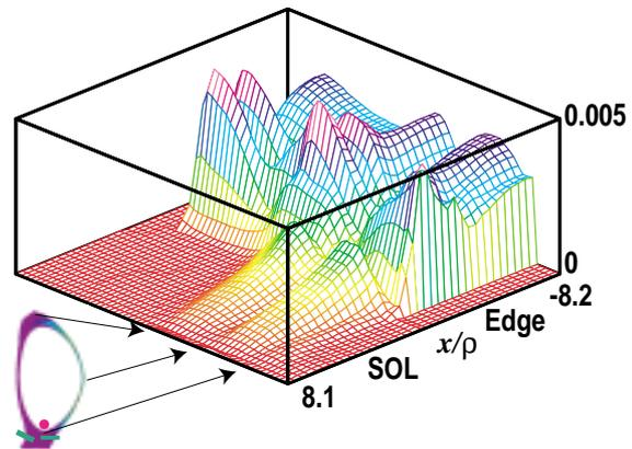
Fig. 5. Contour plot of the electrostatic potential vs. the normalized radial ( $x$ ) and poloidal coordinates, in the linear phase of a BOUT simulation with current.
