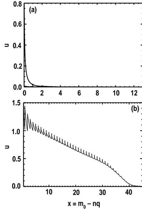
Fig. 3. Radial mode displacement ( $u$ ) in: (a) the moderate squareness case ( $\delta_2 = 0.05$ ),  $\Delta = 0.05$ , (b) the high squareness case ( $\delta_2 = 0.5$ ),  $\Delta = 0.05$ .  $x = m_{0vac} - nq$  is a measure of radial location which increases from zero at the innermost vacuum rational surface to  $\sim 40$  at the top of the H-mode pedestal.
