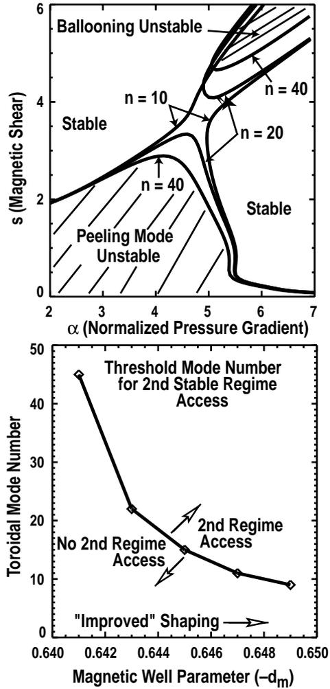
Fig. 2. (a) Stability boundaries of  $s$ - $\alpha$  equilibria for coupled peeling/ballooning modes at  $n=10,20,40$ ,  $d_m = -0.645$ . (b) Calculated marginal value of  $n$  for second stability access, as a function of the magnetic well parameter ( $d_m$ ).
