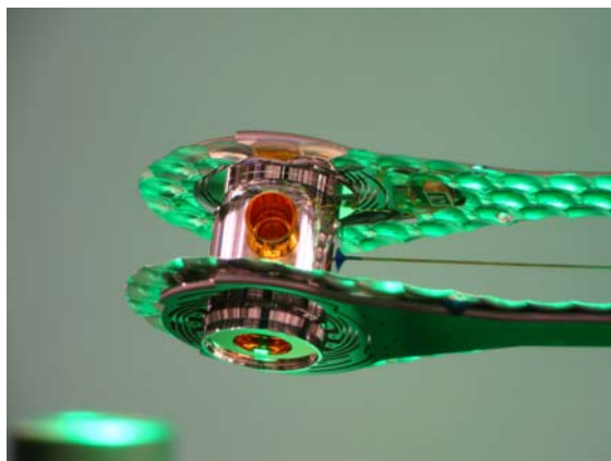
Fig. 3-9. A keyhole target assembly used in shock timing experiments at NIF
