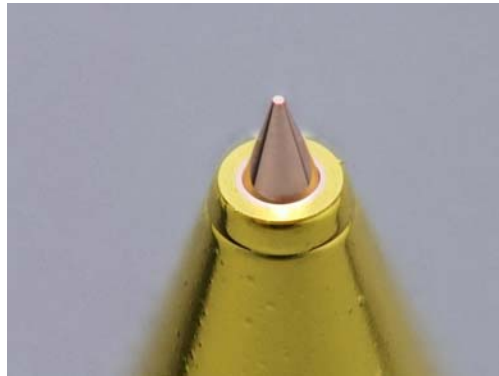
Fig. 3-2. A copper cone, replacing the usual gold cone, was made for fast ignition experiments.
