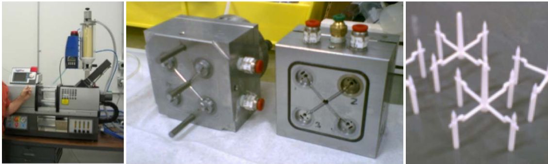
Fig. 7-1. On the left is the injection mold machine, in the center is the four cavity mold for cone mandrels (mold face is 75 x75 mm), on the right are polystyrene mandrels as ejected from the mold, with runners still attached. Each mandrel is \text{Ø}3.2 \times 34.3 mm long.
