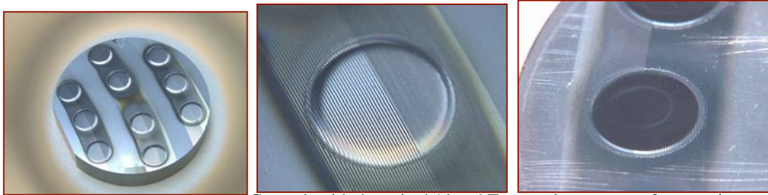
Fig. 7-22. Shown here is the Cu puck with deposited Al and Ta at various stages of processing.
