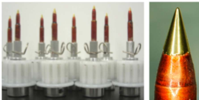
Fig. 7-2. Left, gold cones still on the photomasked, injection molded mandrels, mounted in electro-plating fixtures. Right, detail of tip. Gold cone height is 2 mm.
