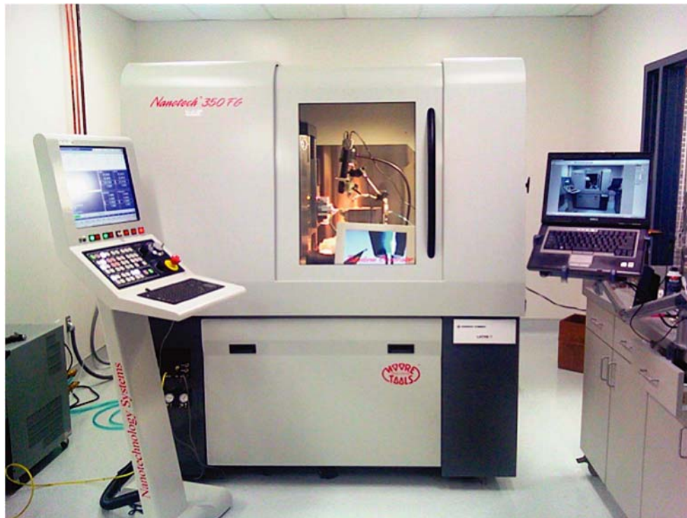
Fig. 2-2. Photograph of the newest addition to the Center for Precision Manufacturing a Moore Nanotech 350 FG, a 5-axis capable high precision diamond turning lathe.
