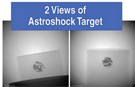
Fig. 5-13. Xradia image of a completed AstroShock target showing the ruby leaded R/F sphere suspended in the R/F foam cylinder.
