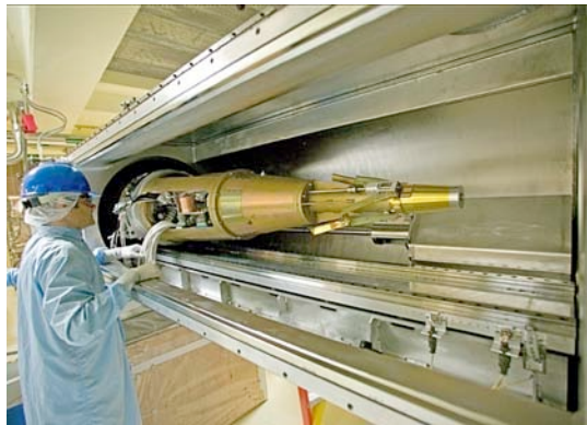
Fig. 4-15. Ignition target inserter cryostat (I-TIC) in the NIF target positioner (TARPOS).
