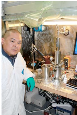
Fig. 2-1. A GDP coater (1 of 9) operated at General Atomics to produce polymer and doped polymer capsules.
