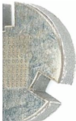
Fig. 3-7. hGXI prototype assembly, 150 \mu\text{m} thick Pt foil containing 10 \mu\text{m} pinholes on 1 mm thick Ta substrate containing 100 \mu\text{m} diameter collimator holes concentrically drilled to less than 3 \mu\text{m} placement accuracy.
