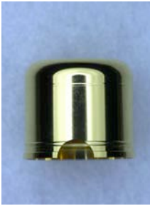
Fig. 4-11. Photograph of the machined hohlraum for the KeyHole target.
