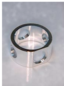
Fig. 4-8. Photograph of the diagnostic band for the KeyHole target.
