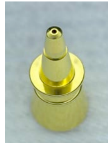
Fig. 4-9. Photograph of the diagnostic gold cone for the KeyHole target.
