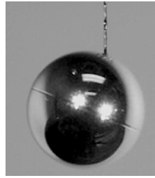
Fig. 5-5. Complete, fully assembled DImE target mounted on stalk at LLE by GA staff.
