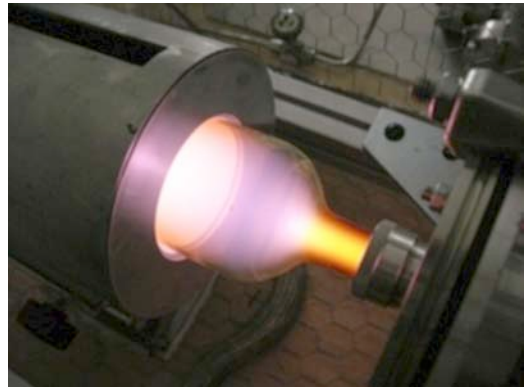
Fig. 2-5. A developmental GDP Coater in operation at GA to coat thin gas retentive layers onto foam capsules.
