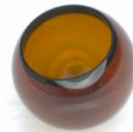
Fig. 4-10. Photograph of the machined capsule for the KeyHole target.
