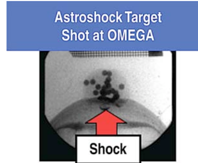
Fig. 5-14. Image of a completed AstroShock target shot on the OMEGA. The image shows the shock as it starts to impact the ruby-loaded R/F foam bead.
