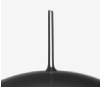
Fig. 3-49. An 11\ \mu\text{m} diam PAMS stalk attached to the mandrel.
