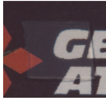
Fig. 3-57. Picture of a ~100 mg/cc alumina aerogel of 0.7 mm thickness.
