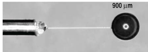
Fig. 4-29. The length of the stainless steel tube serves as a reservoir increasing the effective volume of gas in the shell for this room temperature OMEGA cryo surrogate.
