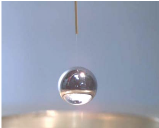
Fig. 3-2. Beryllium shell with fill tube.
