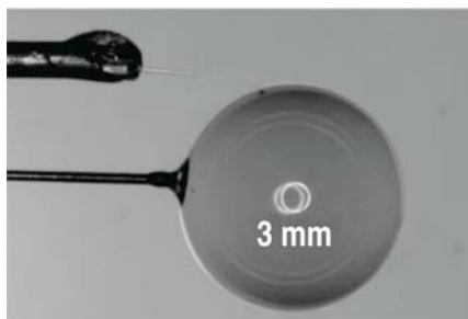
Fig. 4-30. The fill tube comes in from the top with a side support stalk attached for the NIF scale CD and RF foam shells.
