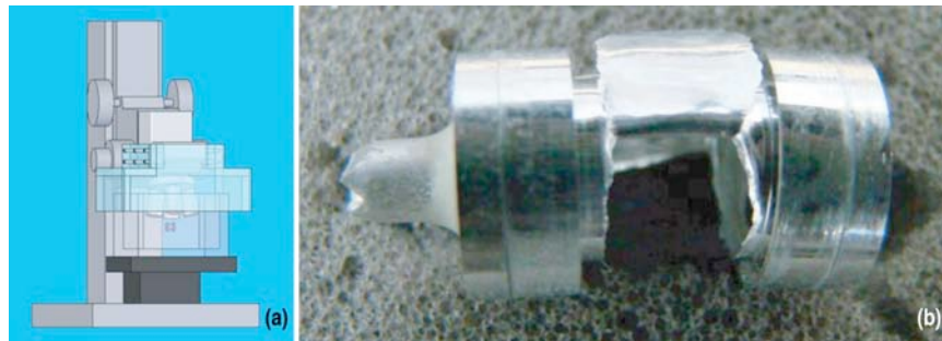
Fig. 6-4. (a) Interference microscope with polycarbonate safety enclosure (colored aqua). (b) A prototype target that catastrophically failed during the pressure testing.
