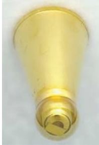
Fig. 3-6. Shock timing cone-in-shell target used to observe the shock-breakout on imploding capsules.
