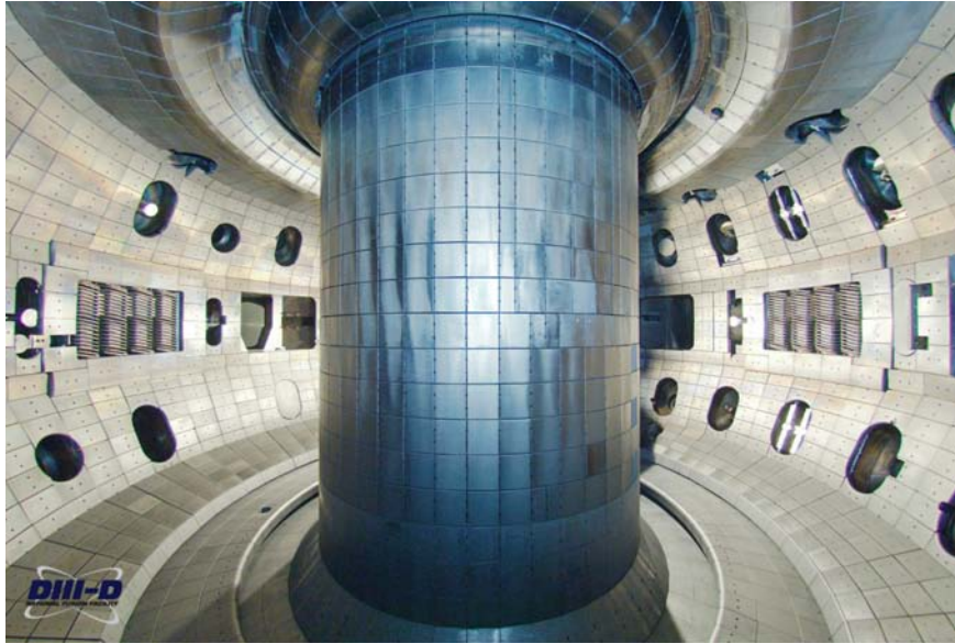
Fig. 8-1. View of the tokamak interior showing some of the internal diagnostics and large port access.
