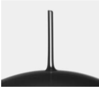
Fig. 3-49. An 11\ \mu\text{m} diam PAMS stalk attached to the mandrel.
