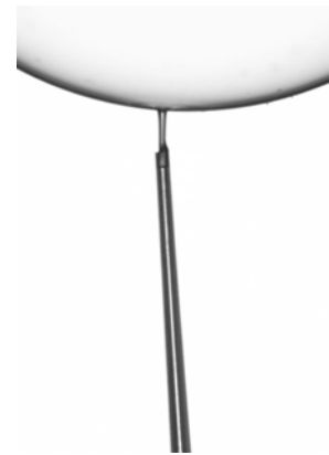
Fig. 3-53. A 3.1-mm-o.d. MFT capsule attached to the supplemental polyimide fill tube. The glue joint is \sim 100 \mu\text{m} from the capsule surface.
