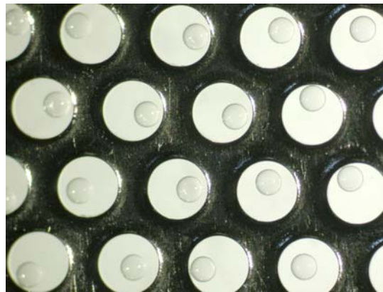
Fig. 3-19. A grid of shells ready for diameter and wall thickness measurements.
