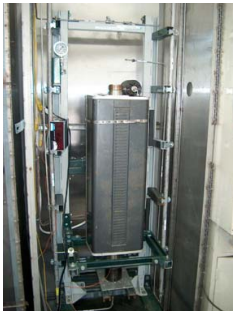
Fig. 6. Test apparatus set up with the pressure vessel tube sitting inside the tube furnace.
