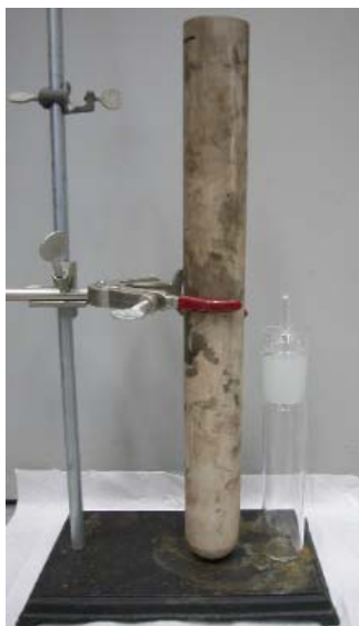
Fig. 9. Mullite tube in which the test cell is located.
