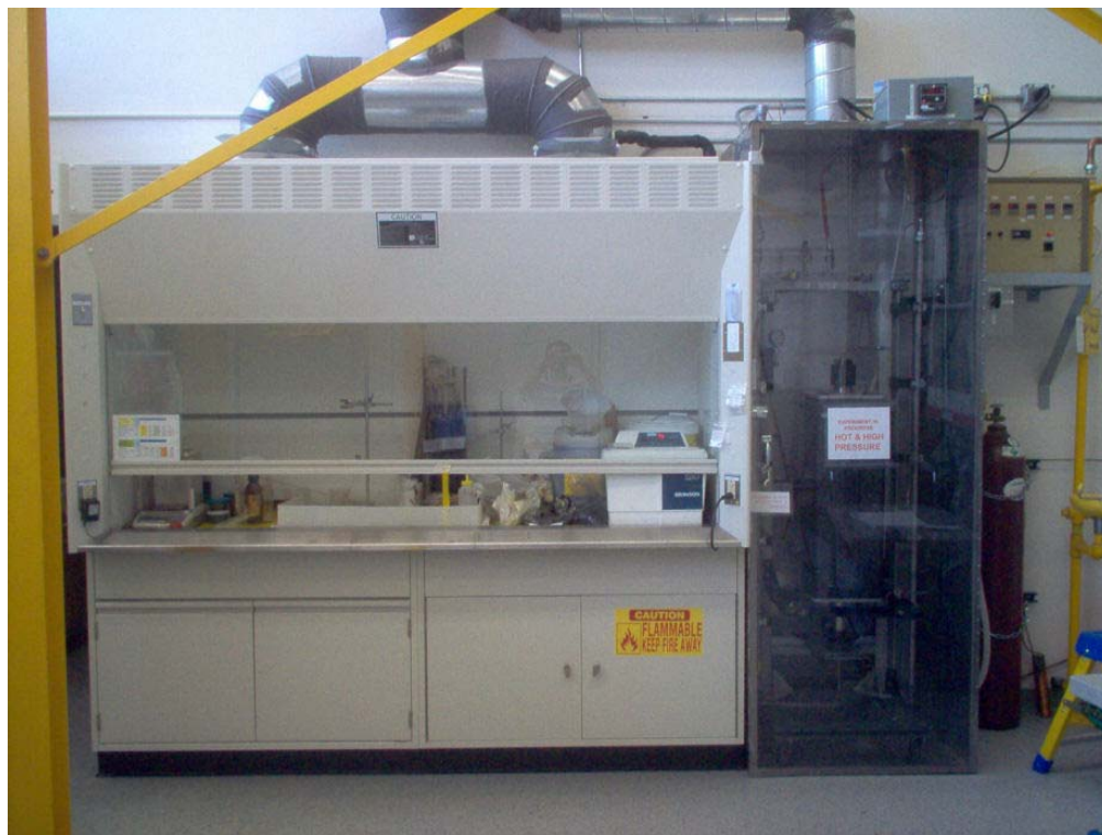
Fig. 11. Immersion corrosion test system enclosure and fume hood.
