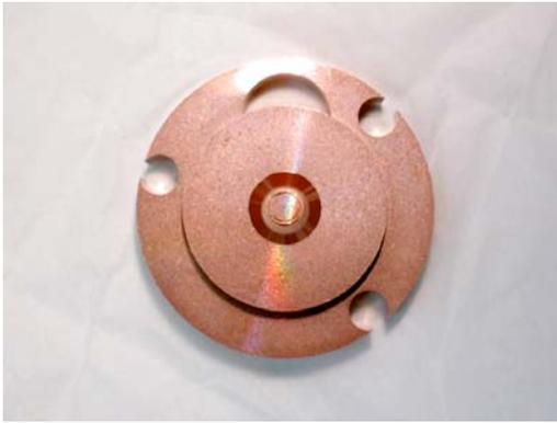
Fig. 9-3. A complex copper fixture to be used in cryogenic double-shell tests.
