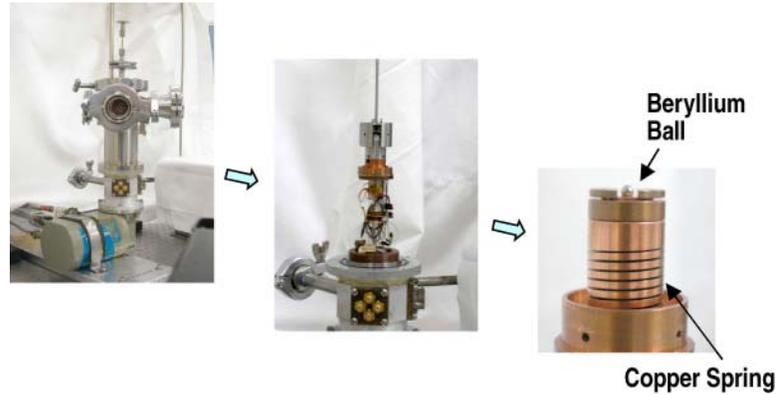
Fig. 15-7. Apparatus for testing capsule to cone seal at 10 to 20 K.
