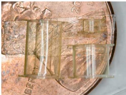
Fig. 2-3. Epoxy cylinders designed to contain gas. They are sitting on a penny. A membrane will be mounted on the flange at the end of each cylinder.
