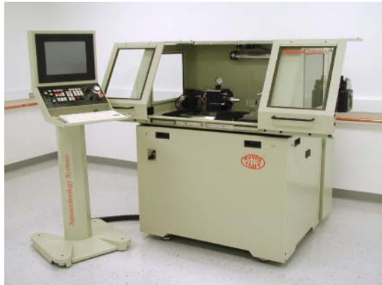
Fig. 22-1. Nanotech 220UPL-HD diamond turning machine.
