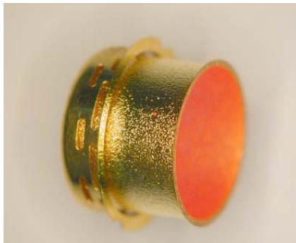
Fig. 2-1. One half of a cryohohlraum. These components are produced in halves and are joined once the capsule is mounted. The inner barrel has been roughened to scatter infrared (IR) radiation, which is used to aid layering of the DT ice in the capsule.
