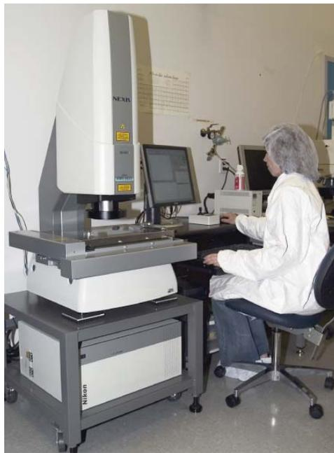
Fig. 8-3. NexIV automated measure scope.
