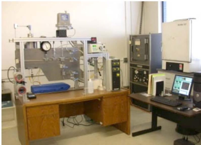
Fig. 6-1. Silica aerogel reactor.
