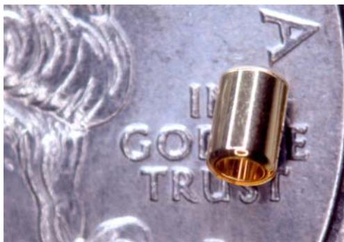
Fig. 2-4. A thin-walled gold hohlraum sitting on a dime. The Au wall of the hohlraum is  $2\ \mu\text{m}$  thick and is reinforced with a  $100\ \mu\text{m}$  thick layer of epoxy.
