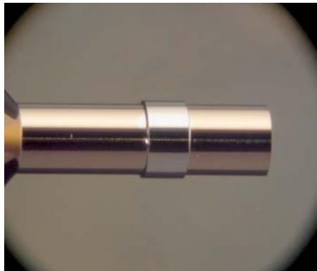
Fig. 7-1. Photomicrograph of aluminum band electroplated on copper mandrel.
