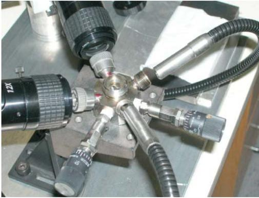
Fig. 19-2. Pressure cell with orthogonal optical access.
