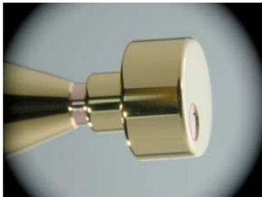
Fig. 9-1. Gold hohlraum on the copper mandrel, which will be dissolved out subsequently. The shape is unusual with two different diameters and an off-axis hole in the face of the large diameter section.
