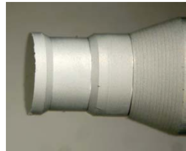
Fig. 3-47. An acrylic mandrel with a successful aluminum coating.
