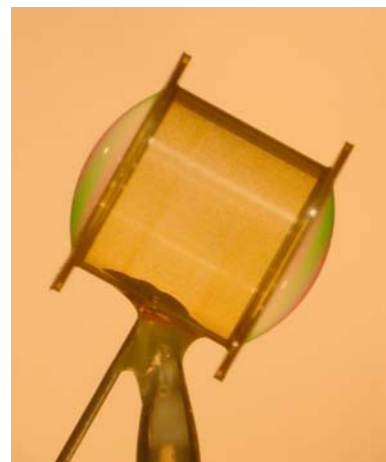
Fig. 3–108. A gas pipe target is a transparent epoxy hohlraum with thin polyimide windows and filled with a specified gas or gas mixture.
