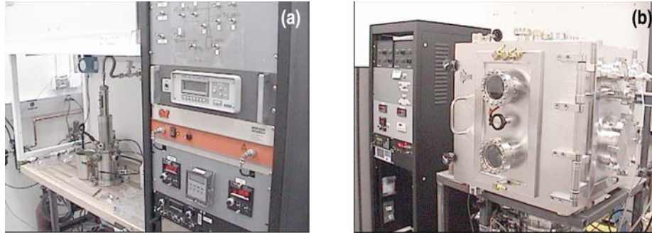
Fig. 3–55. (a) New GDP coater (b) new sputter coater assembled using EQU-03 tasks to reduce production bottlenecks associated with this equipment.
