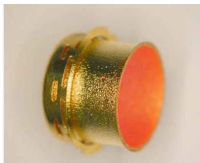
Fig. 3–28. One-half of a cryogenic hohlraum.
