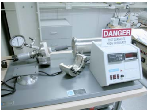
Fig. 3–74. The Hoppe glass shell Parr oven is designed to operate at up to 1100°C and pressures up to 10 atm at temperature.
