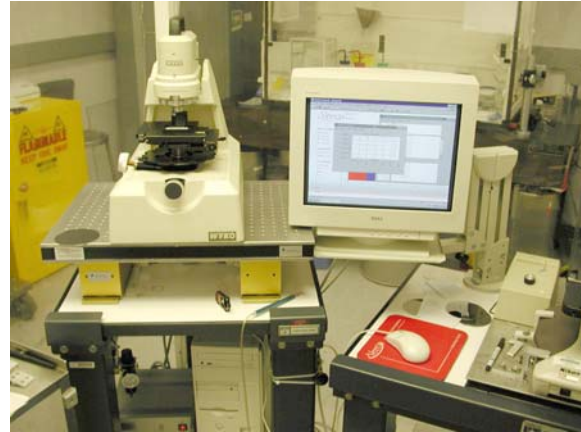
Fig. 3-93. Our Veeco RST-500 scanning surface profilometer is used to measure the surface of complex objects.
