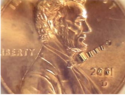
Fig. 3–32. A set of gold cups in varying sizes.
