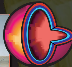
Multiple GDP (Glow Discharge Polymer) Layers Doped with Si, Ge, Ti, Cl, Cu, or D
