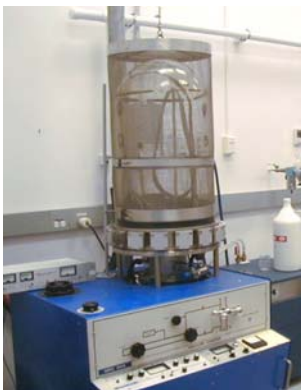
Fig. 3-84. The evaporative coater is used primarily for aluminum or gold coatings with thickness greater than 1000Å.
