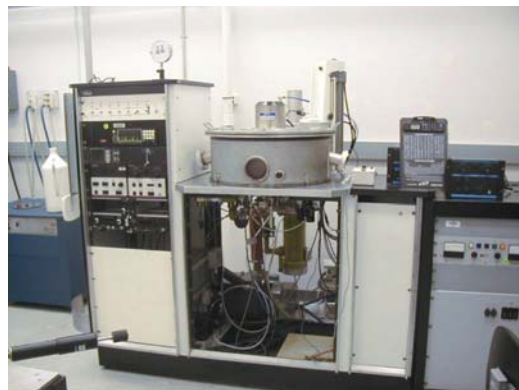
Fig. 3-85. Sputter coating facility at Schafer.
