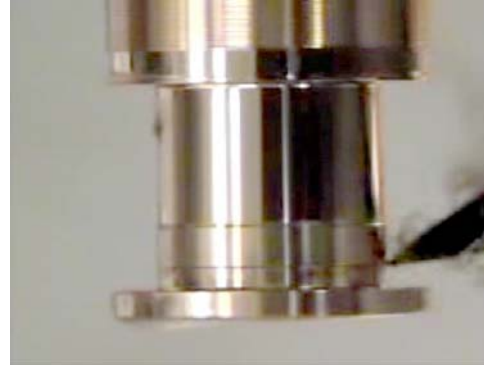
Fig. 3-42. Shaping the front of a copper mandrel. Note the different tool orientation from that shown in Fig. 3-39.
