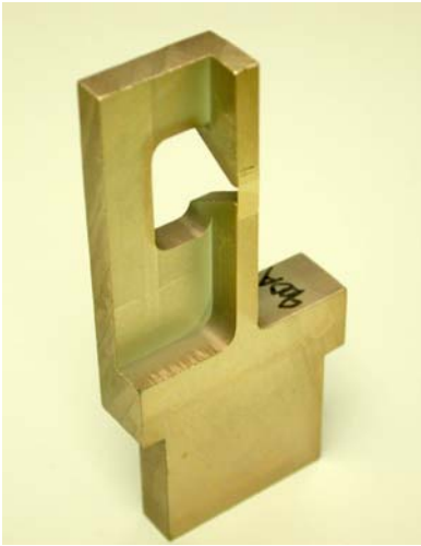
Fig. 3–79. Nike target frame with gold-coated polymer film target.
