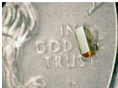
Fig. 3–29. Square cylinder with copper leached out.
