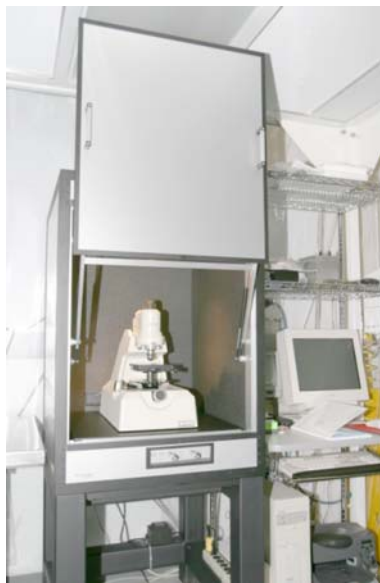
Fig. 3-95. Vibration isolation system.
