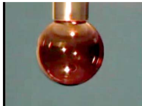
Fig. 3–75. Droplet of PVA resulting from the original spin-coating technique developed for SNL capsule production.
