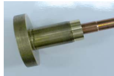
Fig. 3–38. The copper mandrel and holder used for making epoxy hohlraums.
