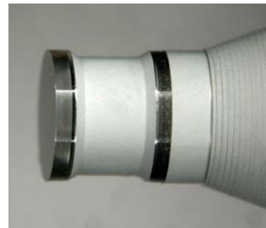
Fig. 3-48. An aluminum coated mandrel after the final machining step.
