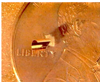
Fig. 3–30. Half-round cylinder with gold leached out.
