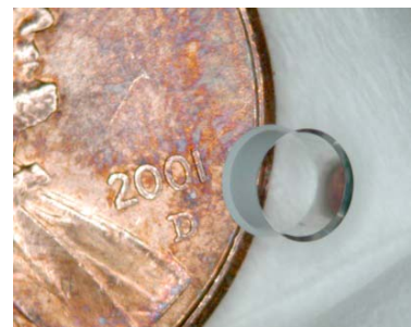
Fig. 3-49. A completed aluminum foil tube.
