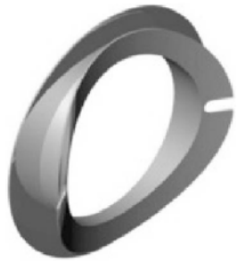
Fig. 3–50. CAD rendering of a window saddle.
