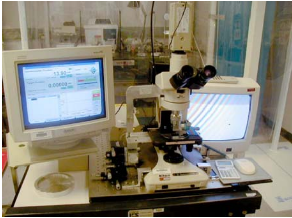
Fig. 3-92. By positioning the fringes from this white light interferometer, focus position and therefore film thickness can be measured precisely.
