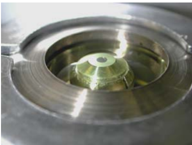
Fig. 3–80. Aluminum CTMs have a film of 1.5\ \mu\text{m} thick Schafer-made polyimide stretched over them and sealed.
