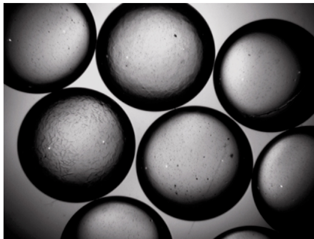
Fig. 6. 3 mm diameter/30 \mu\text{m} wall polystyrene targets made in ME laboratory.
