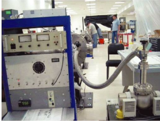
Propellant valve power supply
