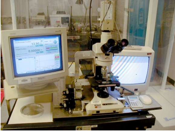
Fig. 3–94. By positioning the fringes from this white light interferometer, focus position and, therefore, film thickness can be measured precisely.
