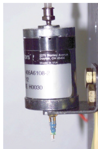
Fig. 3–77. A hole was drilled through the rotor of a small 12-V dc motor so that a vacuum line could be attached to hold a 2-mm GDP shell to the other end of the rotor.
