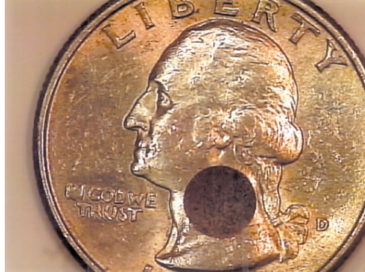
Fig. 3–33. A gold disk 5 mm in diameter and 1.0 mm thick. The surface is very smooth.
