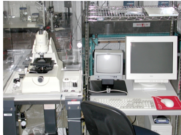
Fig. 3–95. Our Veeco RST–500 scanning surface profilometer is used to measure the surface of complex objects.
