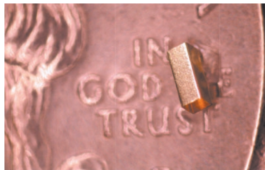
Fig. 3–28. A 0.6 mm square gold cylinder that is 2 mm long. The wall thickness is 25 \mu\text{m} .
