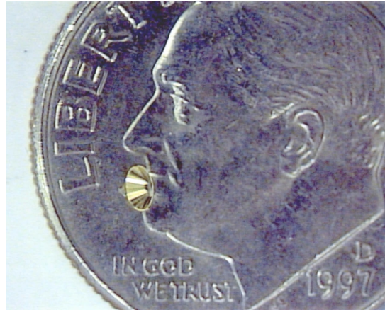
Fig. 3-30. A small truncated gold cone used as part of an ICF target component. The cone is sitting on a dime.
