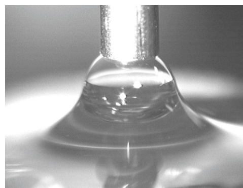
Fig. 3–78. Spinning the shell while it is withdrawn from a solution of PVA causes the PVA to redistribute itself uniformly around the axis of rotation. The shell takes about 10 minutes to dry while it spins.
