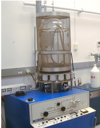
Fig. 3-86. The evaporative coater is used primarily for aluminum or gold coatings with thickness greater than 1000\text{\AA} .
