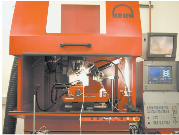
Fig. 3–34. Photograph of the KERN five-axis micromill.
