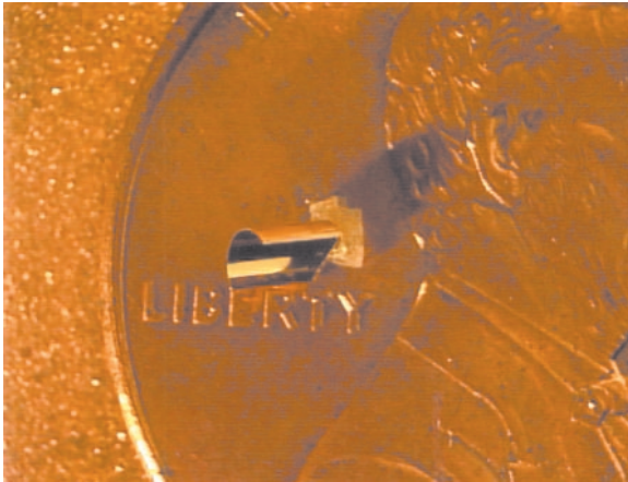
Fig. 3-29. A half round gold cylinder. The diameter is 1.6 mm; the length is 2 mm; and, the wall thickness is 25 \mu m.
