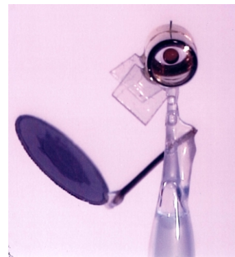
Fig. 3–108. An OMEGA-type target with a capsule-containing hohlraum oriented towards a circular pinhole array.
