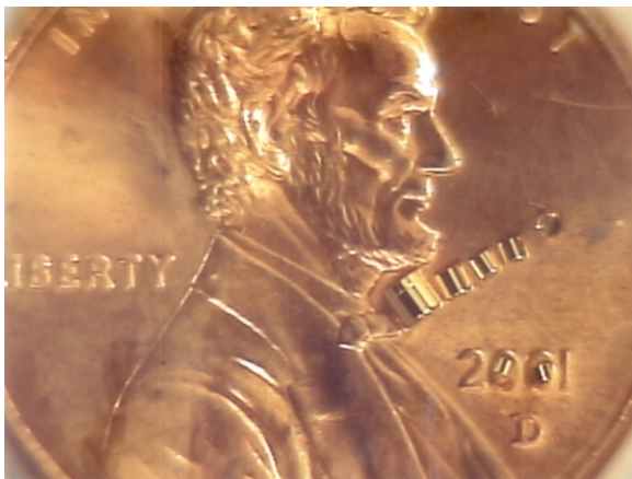
Fig. 3-31. A set of gold cups of different diameters and lengths. The diameters range from 0.64 to 0.16 mm and the lengths range from 0.6 to 0.15 mm.
