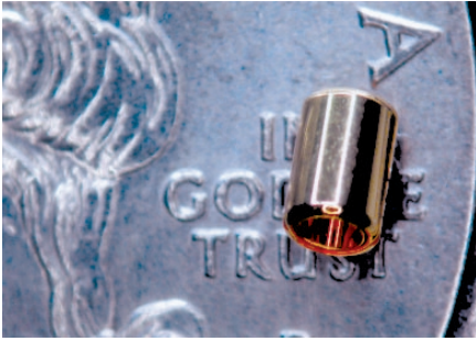
Fig. 3–26. A 1.6 mm diameter hohlraum which is 2.55 mm long with a wall made up of 2 \mu\text{m} of gold and 100 \mu\text{m} of epoxy.
