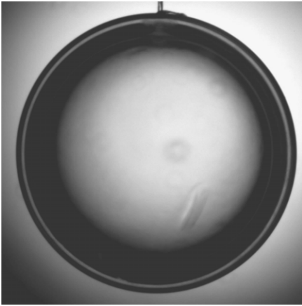
Fig. 3–19. Shadowgraph of a 125 \mu\text{m} layer inside of a 2 mm diameter 40 \mu\text{m} thick polymer capsule with a fill tube. The ice layer is the narrow white band just inside of the capsule edge. The layer roughness is 1.1 \mu\text{m} rms over modes 1 to 50. It is expected that removal of the fill tube and better centering of the shell will reduce the rms substantially by removing a source of low mode defects. The defect in the lower right part of the capsule is left over from where the slowly grown surface met during initial formation. The small circular defects are out of focus dust particles on the polymer capsule surface.
