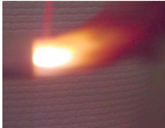
Fig. 25. Electrical ignition of Sn pellet during wire ignition testing.
