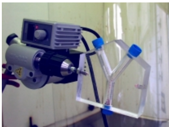
Fig. 7. V-mixer used in mixing tests.
