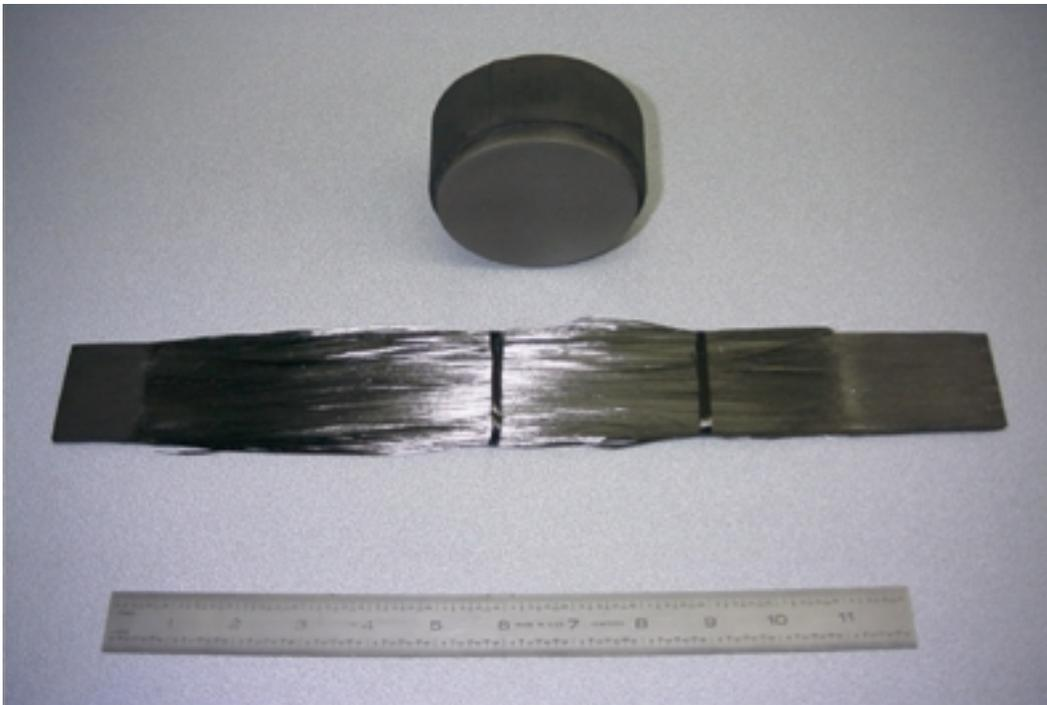
*Fig. 9.1. Photograph of the prototype graded CVD/CFC mirror and flexible carbon fiber bundle under development for use in advanced long pulse ECH launcher mirrors.*
