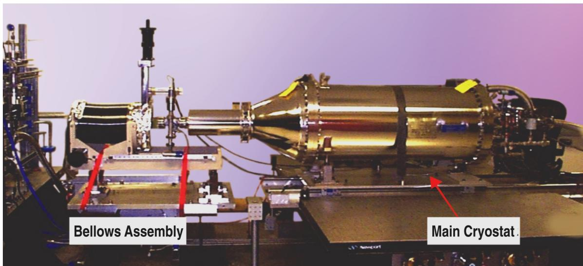
Fig. 3–2. Filled targets will be moved from the bellows assembly into the main cryostat. IR layering of the fuel takes place inside the main cryostat which holds the temperature constant to  $\pm 1$  mK.
