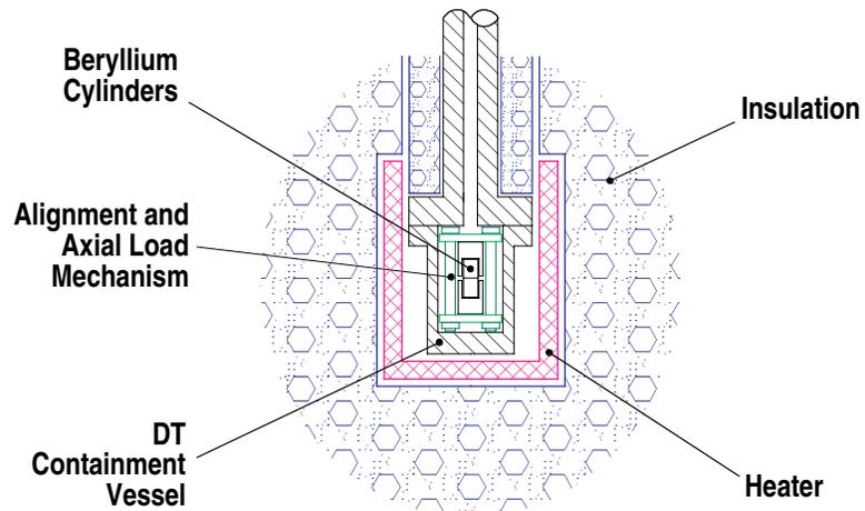
Fig. 3-12. Inner components of the Be Capsule Fill Station heat, compress, and seal together the ends of two Be cylinders that have hollowed hemispherical cavities machined into them. Helium on the outside, maintained at the same pressure as DT on the inside, keeps the containment vessel from exploding.
