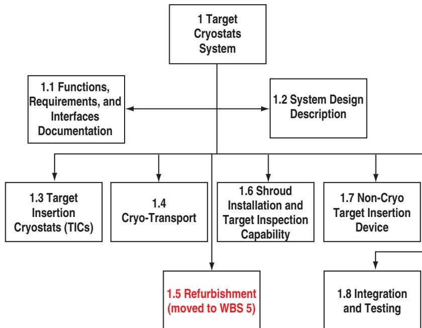
Fig. 3-6. The WBS for the Target Cryostats System.
