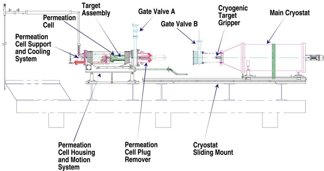
Fig. 3–1. The assembly layout of the D<sub>2</sub>TS.
