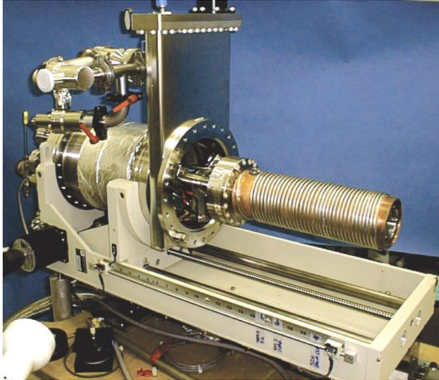
Fig. 3–4. The permeation cell for a system nearly identical to that of D<sub>2</sub>TS (cell shown here with the bellows withdrawn) has passed pressure proof and leak tests up to 15,000 psi. The cell has been cooled to 16 K.
