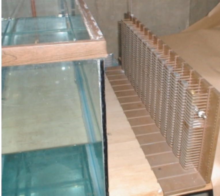
Fig. 9.1. GA combline antenna mockup and water load.
