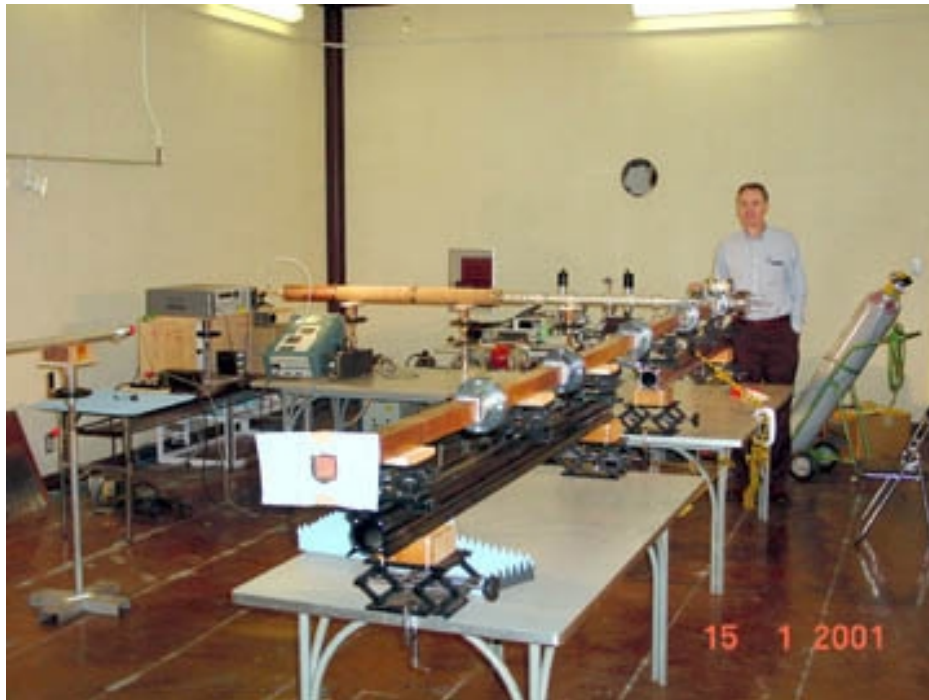
Fig. 9.2. Remotely steerable launcher apparatus in low power testing at JAERI.
