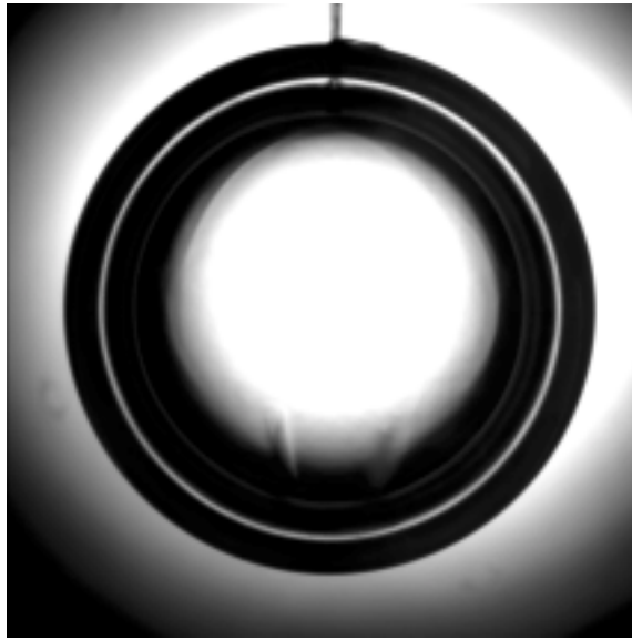
Fig. 5.2-3. CCD image of a D-T solid layer inside a 2-mm plastic sphere. (Image and Gaussian data provided by J. Sater and LLNL.)
