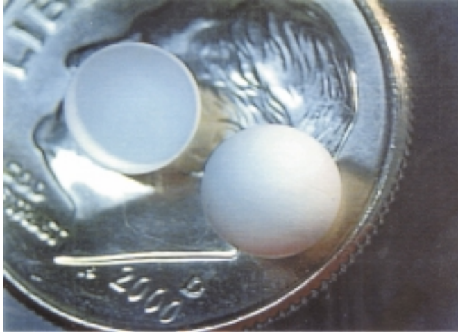
Fig. 3.3-1. A 5-mm diam PS foam hemishell rests upon FDR's cheekbone, while two such hemishells, glued together, rest behind his ear. The foam density is about 250 \text{ mg/cm}^3 and the wall thickness is 160 \text{ }\mu\text{m} . The GDP coating has not yet been applied to this shell.
