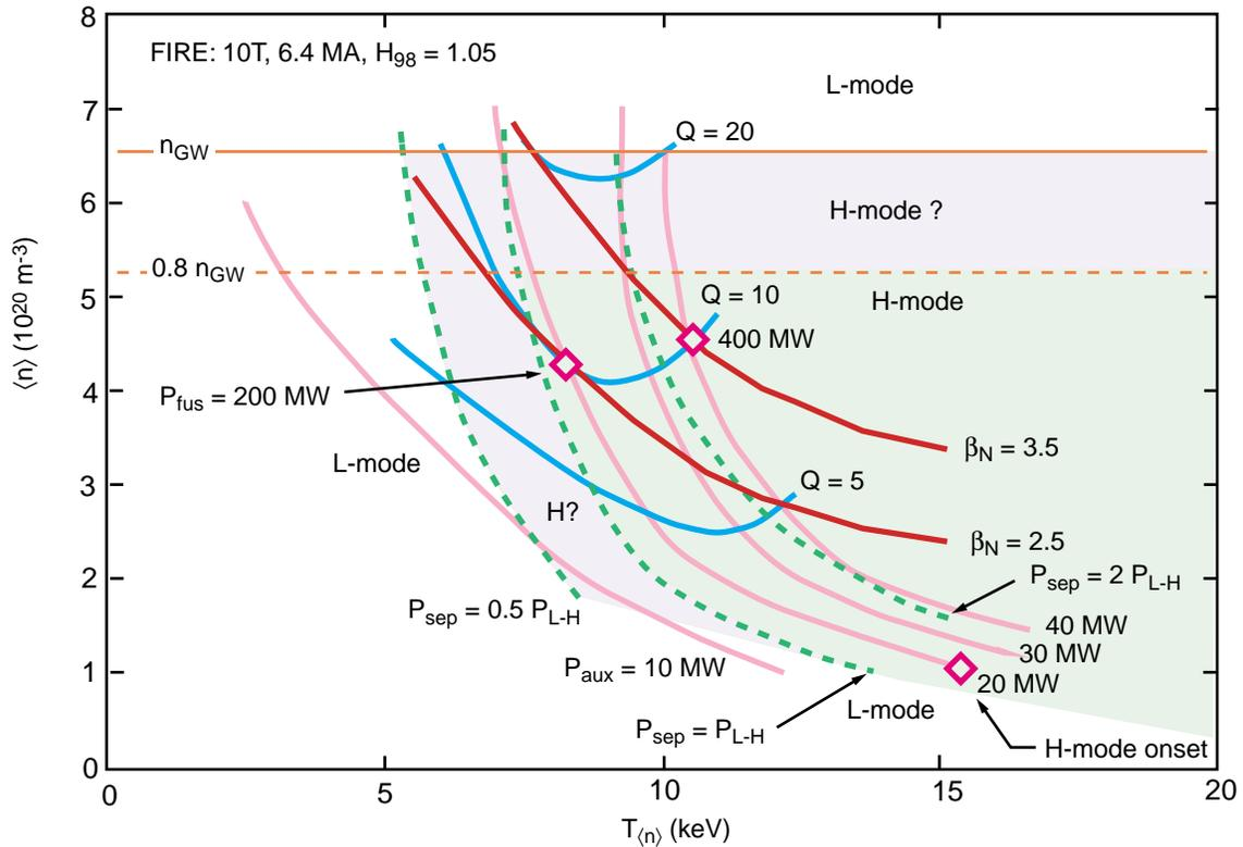
Fig. 5-1. FIRE plasma density/temperature plot with H-mode and L-mode domains indicated. The final FIRE operation point at  $4 \times 10^{20} \text{ m}^{-3}$  density and average temperature of 8.5 keV lies near the lower density bound of the sustainable H-mode domain.
