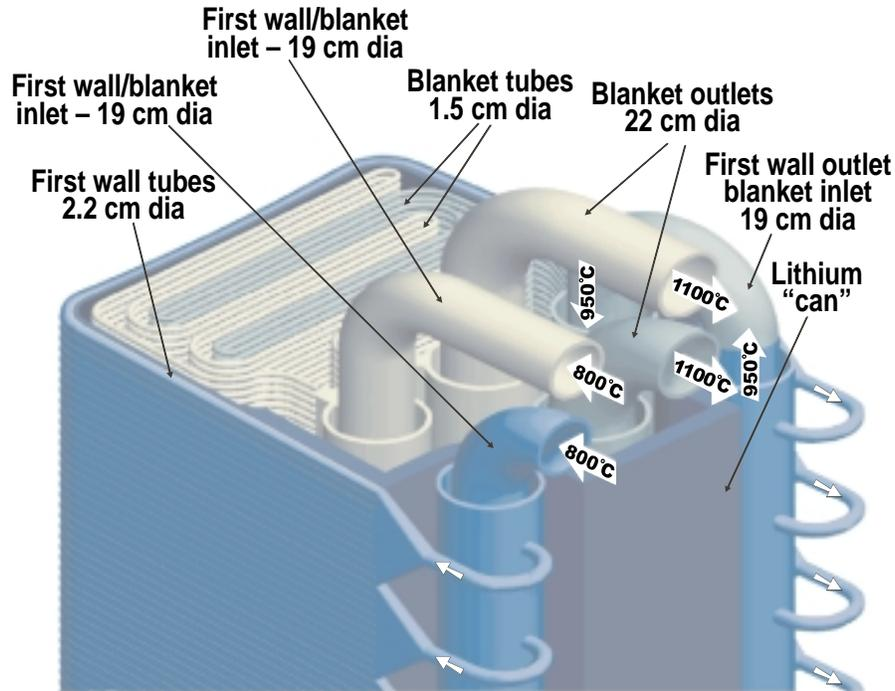
Fig. 4-1. APEX helium-cooled blanket concept. One of three “cans” per outboard sector shown with top removed.
