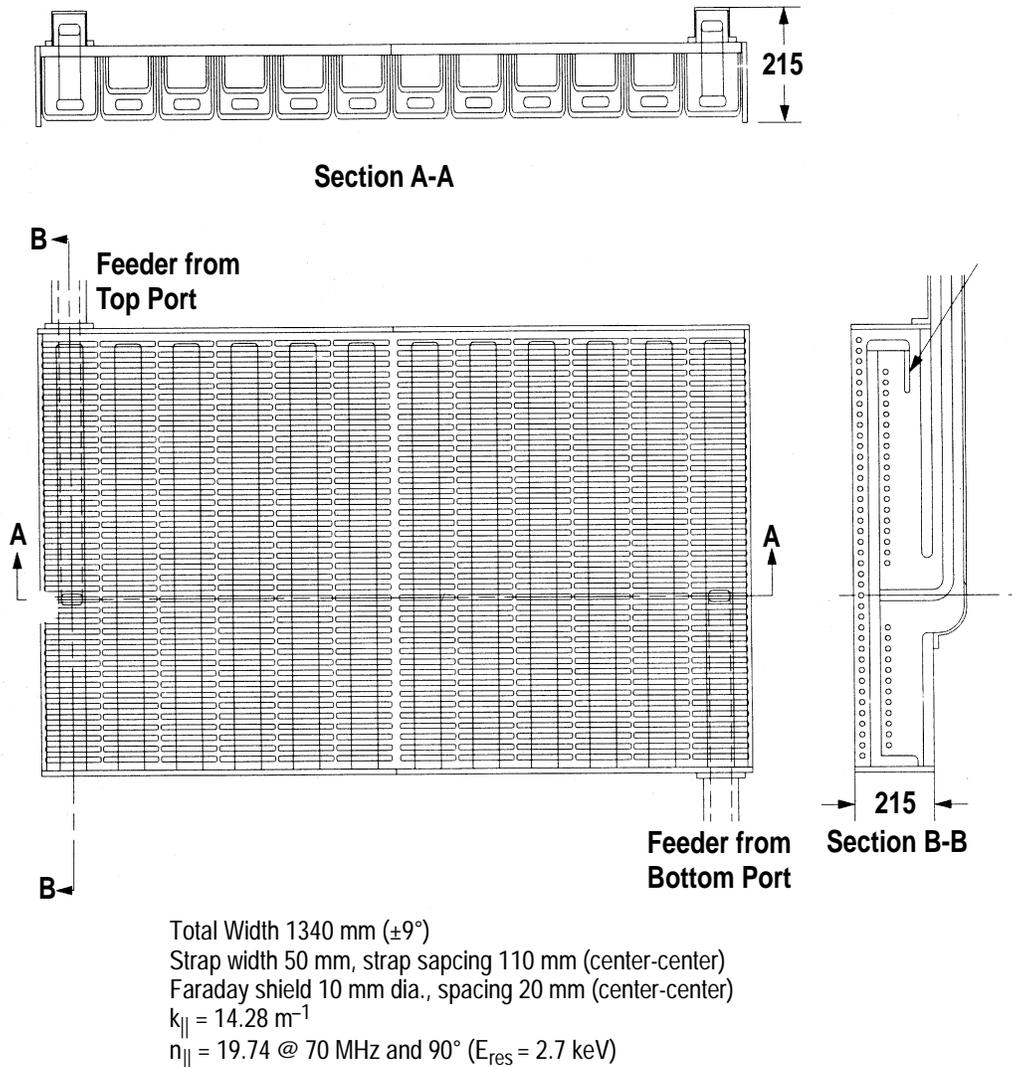
*Fig. 9-1. LHD 12 strap combline antenna.*
