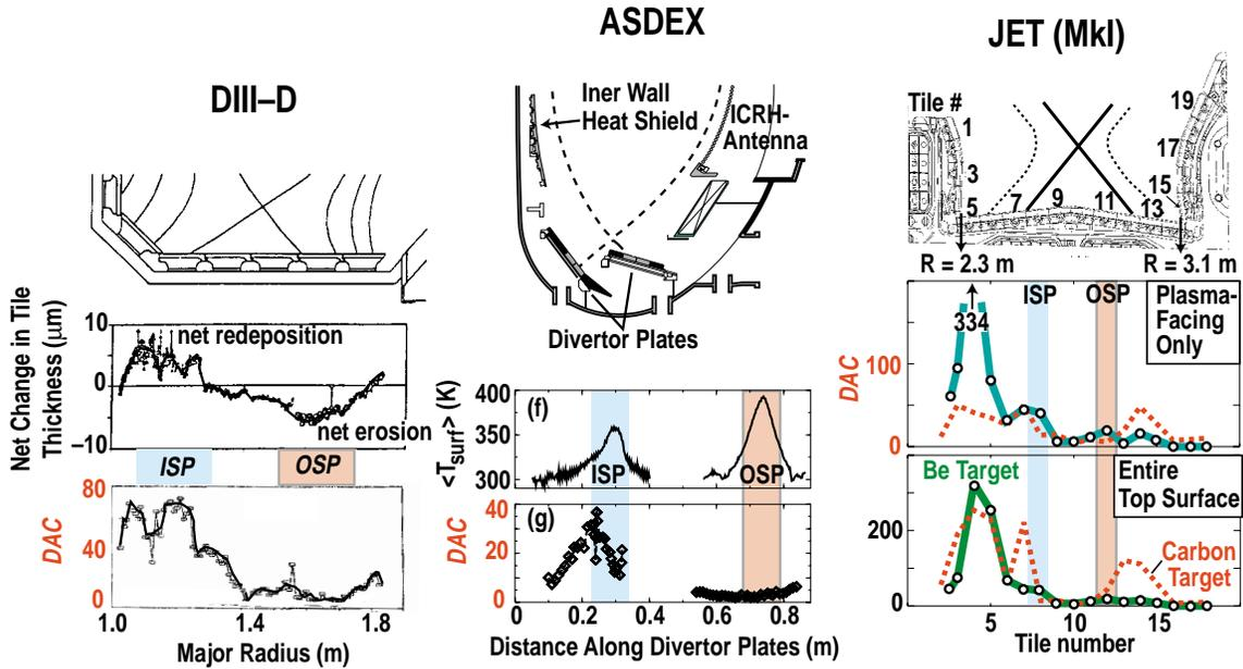
**DAC:** Trapped D concentration over ~1 year of tokamak operation, primarily attached outer divertor operation
