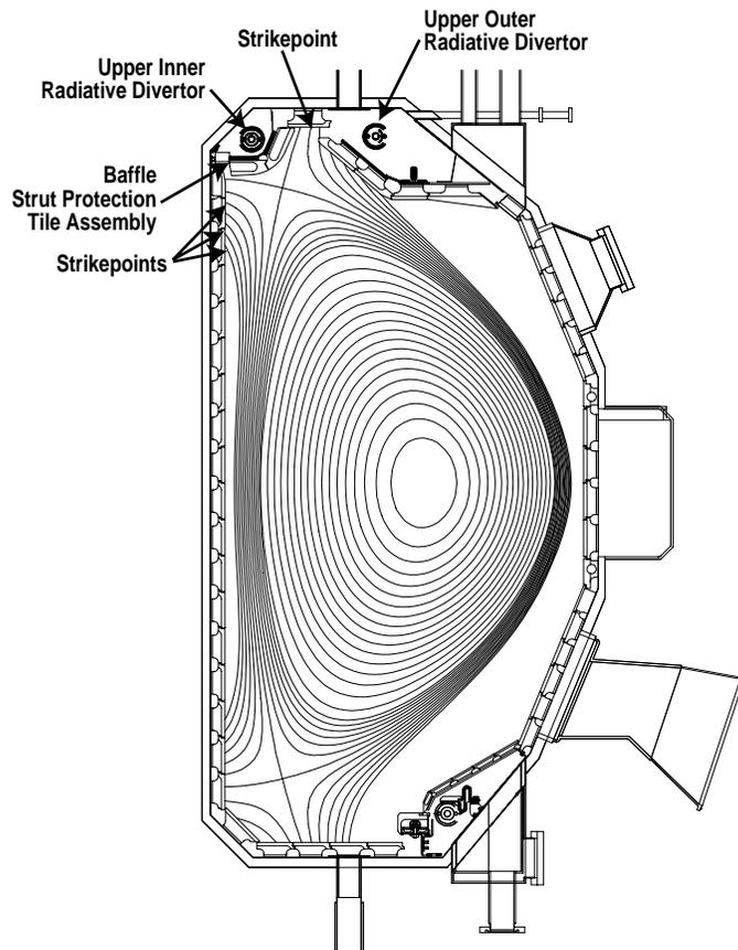
Fig. 8-2. The strut protection tile assemblies are located in the upper inner radiative divertor.
