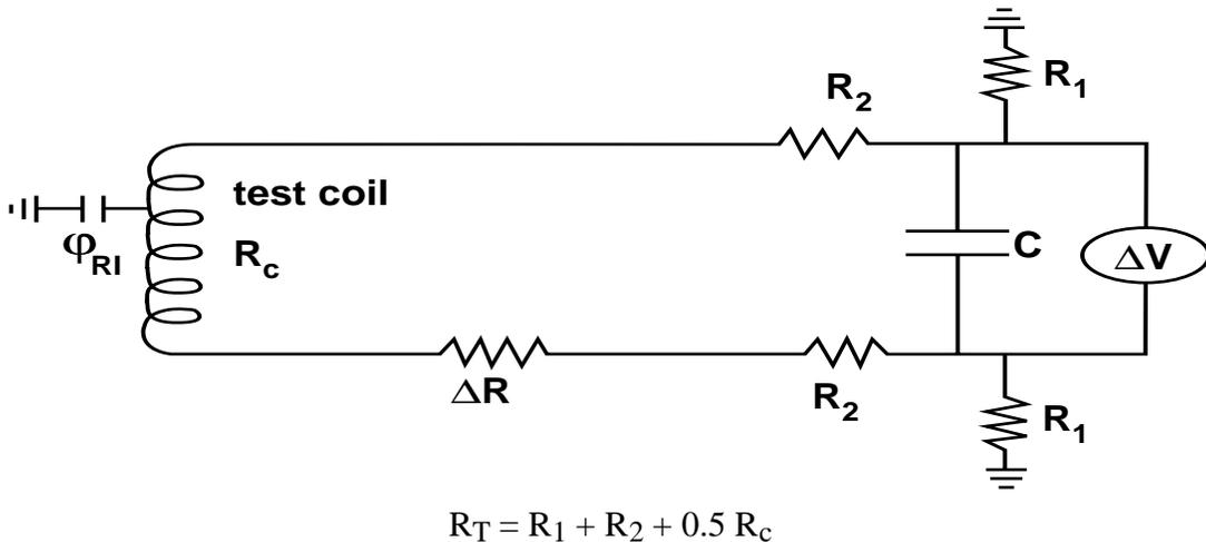
Fig. 7-1. Imbalance in electrical resistance across integrator leads to drift when RIEMF present.
