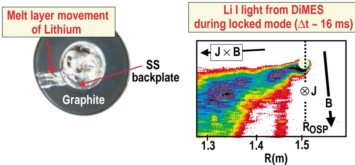
Fig. 6-1. First exposure of a Li sample in DIII-D.
