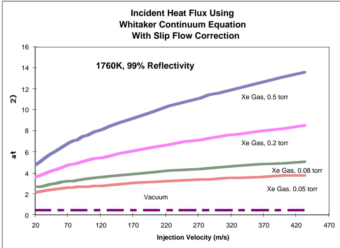
Fig. 10-1. Calculated heat flux on target under varying chamber conditions and injection velocities.
