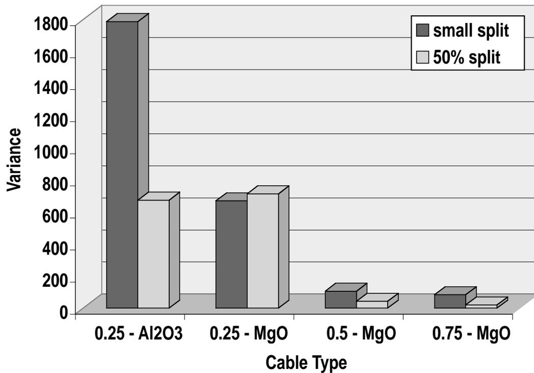
Fig. 7-2. Variance of drift by cable type and compensation method.
