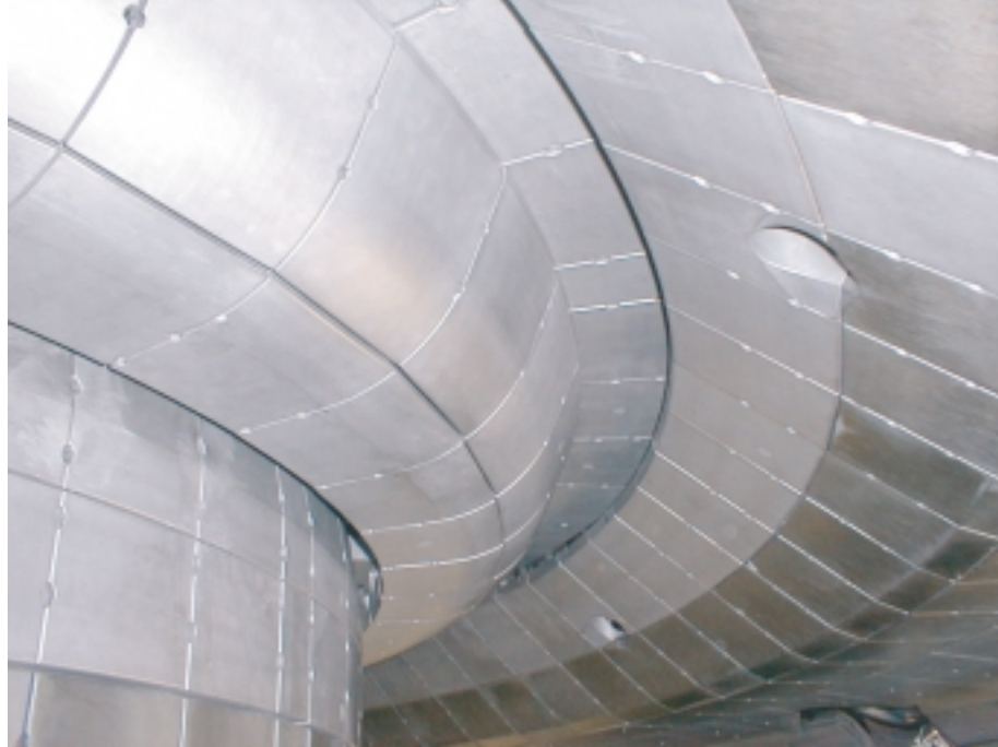
Fig. 4.2-2. Upper outer and inner radiative divertors.
