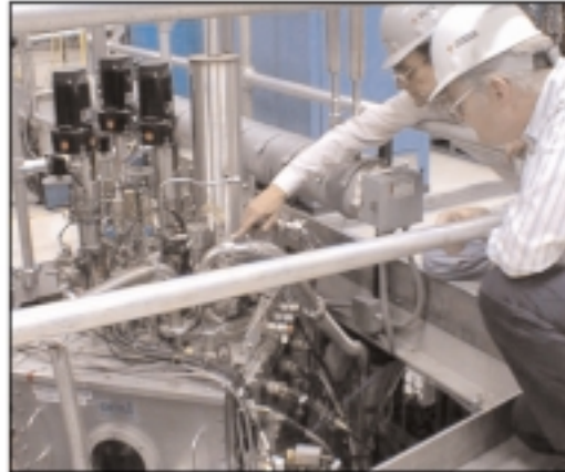
The Oak Ridge pellet injector on the DIII-D tokamak injects pea-size hydrogen ice pellets.
