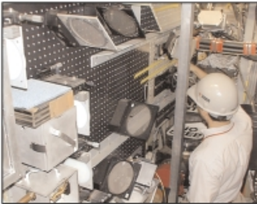
The laser diagnostic instrument developed at UCLA to characterize turbulence. This technology is also applicable for molecular spectroscopy and radiometric imaging from space.
